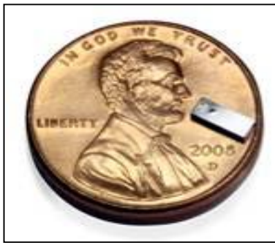
Mini-Pacemaker for Implantation into Heart muscle (Source: Medtronic)
