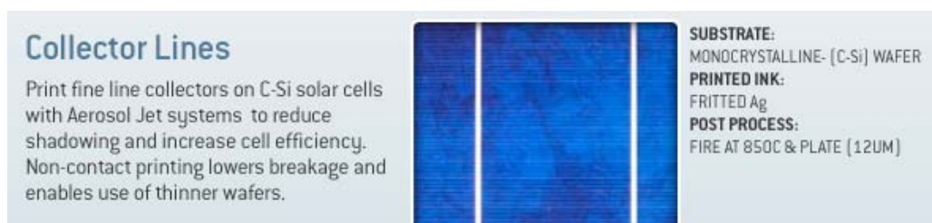
Fig. 60 Collector Lines produced through printing (Source: Optomec)
