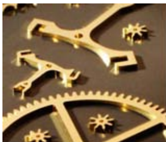
Fig. 67 Beam based production of Ultra precision part for luxury watches (source Microworks)
