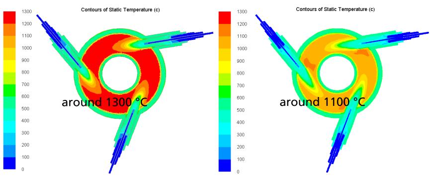
Temperature distribution in the combustion chamber during the combustion of natural gas (left) and of product gas (right)
