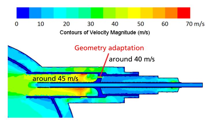
Flow velocity in the injector with modified nozzle holes during the combustion of product gas
