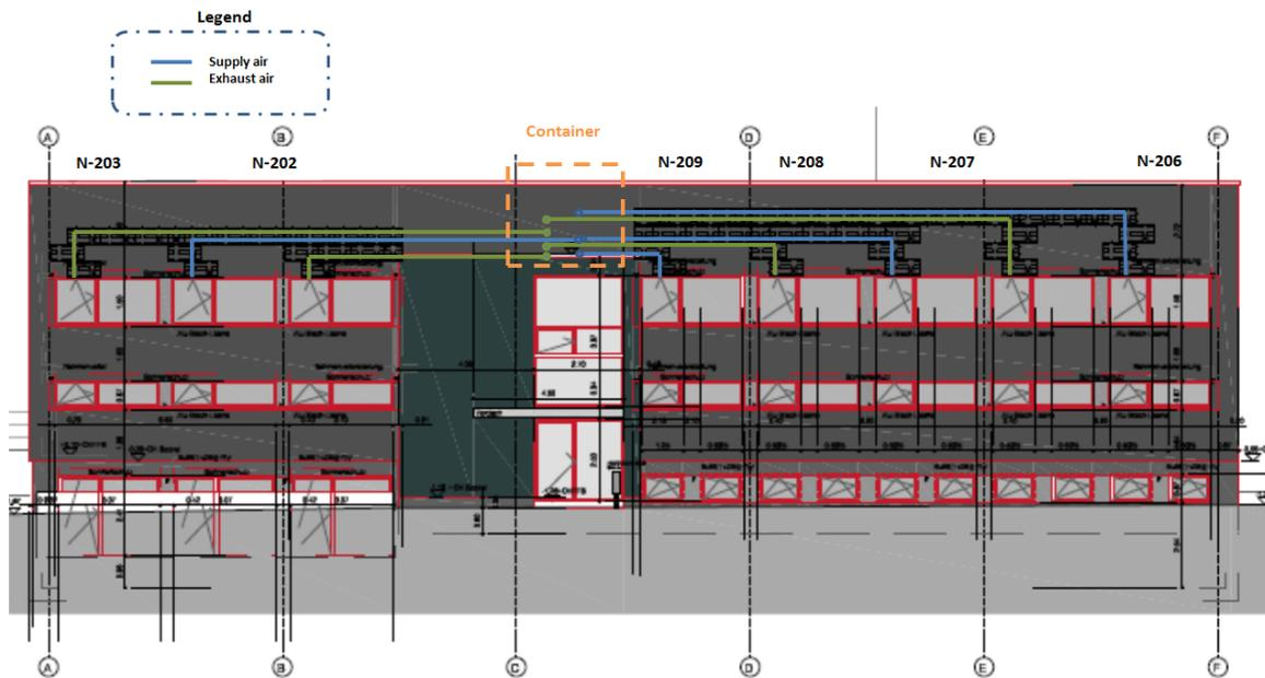
Figure 2 Renovated façade with air ducts paths
