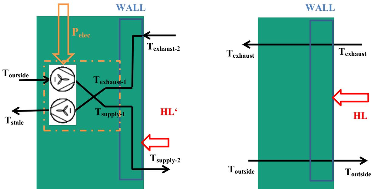
Figure 4 Thermal balances of the analysed system (left) and reference case (right)
