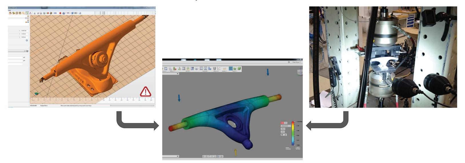
■ This Data was used to check the overall stiffness after the creation of the lattice
