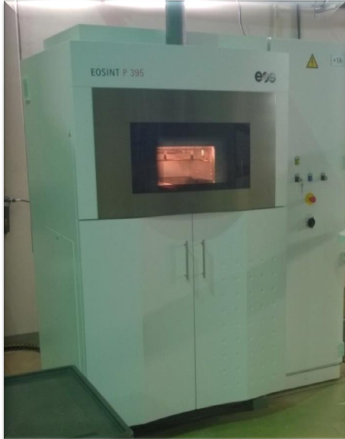
EOS P395 - laser sintering plant for plastic material
