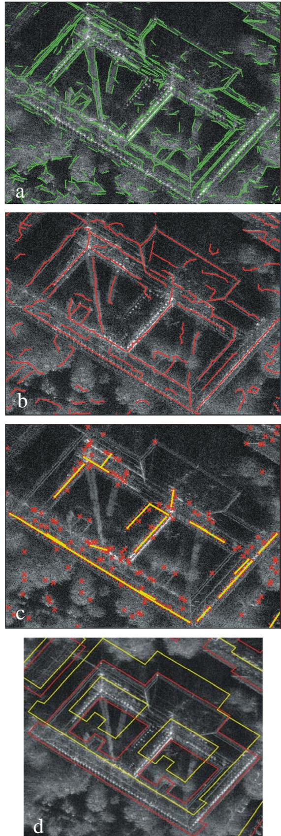
Fig 2. a) Burns edge segmentation, b) Steger line segmentation, c) dominant point scatterers (red) and grouped linear scatterers (yellow), d) SAR image superimposed with building footprints (yellow) and predicted roof position (red).
