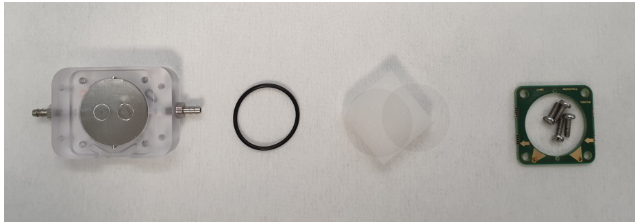
Figure 26: Prepreparation of the samples beginning from the left: micropump without actuator, Sealing ring, glass lip, screw fastening
