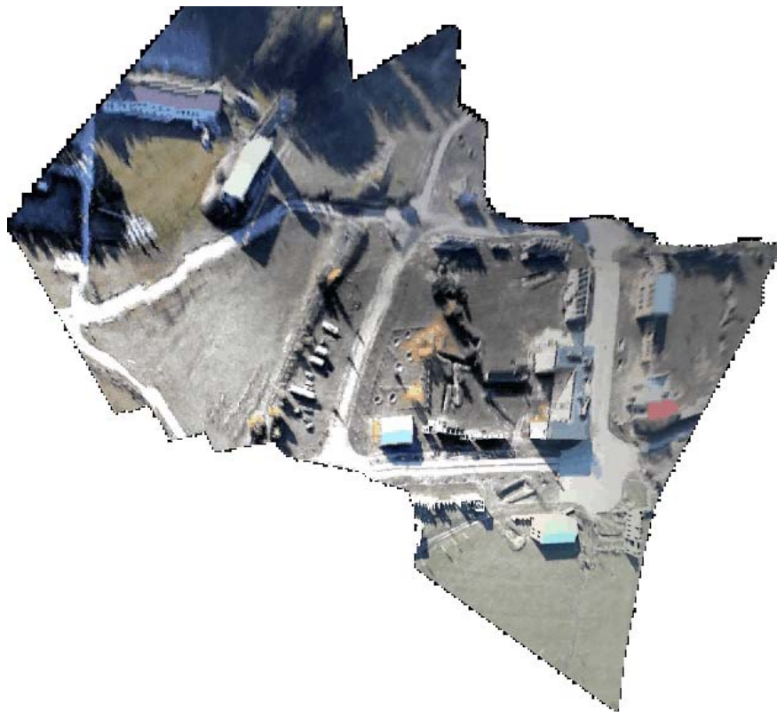
Figure 10: Mosaic created by projection of image sequence onto the ground.
