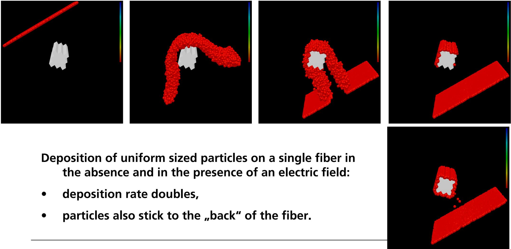
Deposition of uniform sized particles on a single fiber in the absence and in the presence of an electric field:
