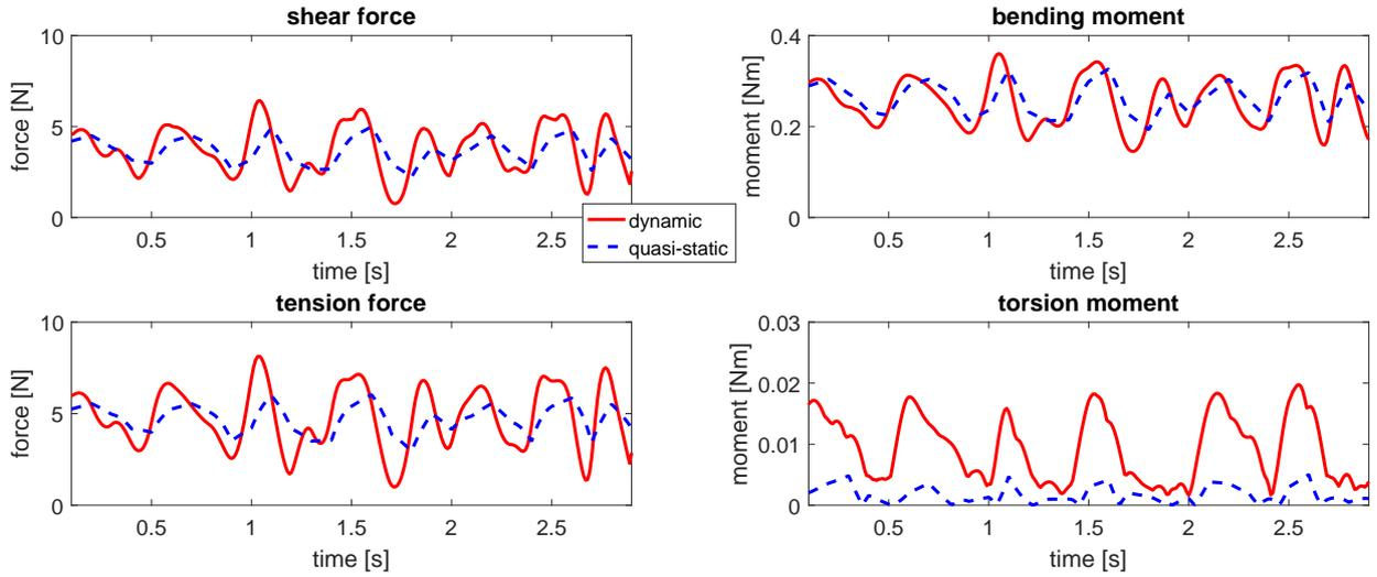
Figure 2: Comparison of simulation results: The maximum values along the cable of shear force, tension force, bending moment and torsion moment are plotted over time for quasistatic (dashed) and dynamic (solid) cable simulation.
