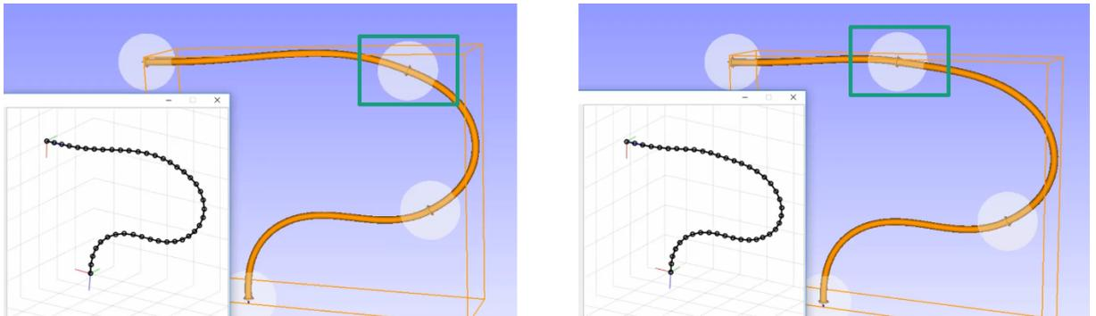
Figure 6: Two mounting variants of cable with four mounting clips. The upper right mounting clip (highlighted by the rectangle) is shifted between the two variants.
