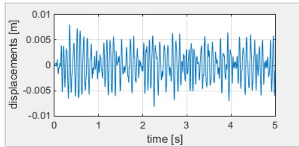
Figure 7: Excitation of the mounting clips, generated by defining its PSD.
