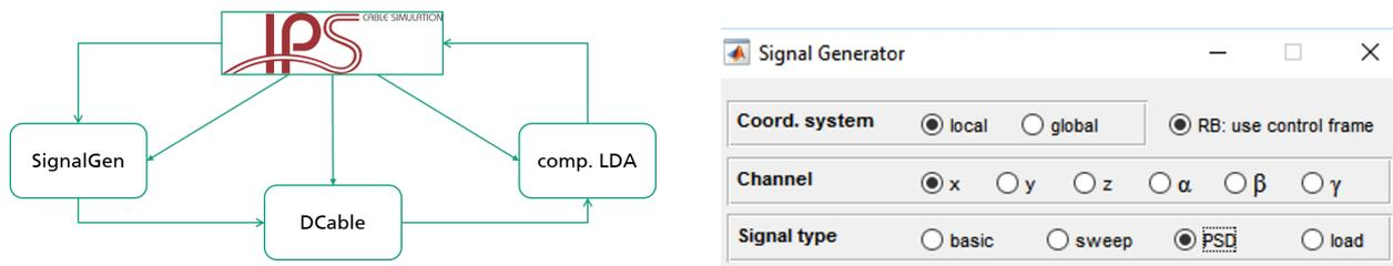
Figure 4: Left: Module overview with *IPS Cable Simulation* as central software tool and the modules *Signal Generator*, *Dynamic Cable Simulation* and the *comparative Load Data Analysis*. Right: Initial mask of the *Signal Generator* with user choice of the coordinate system, the channel and the signal type.
