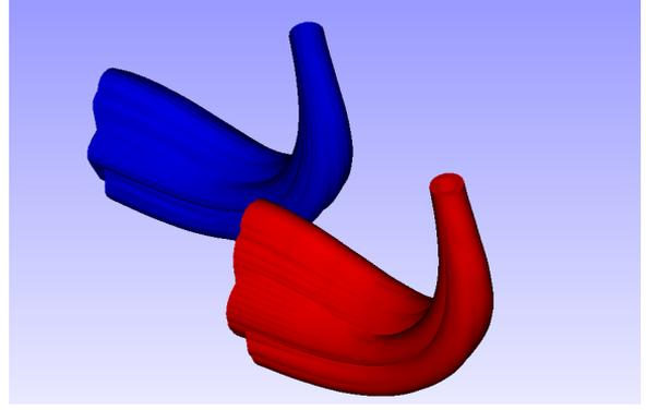
Figure 1: Left: Engine compartment with hose, color-coded with its bending moment. Right: Motion volume of quasistatic (blue) and dynamic (red) simulation.
