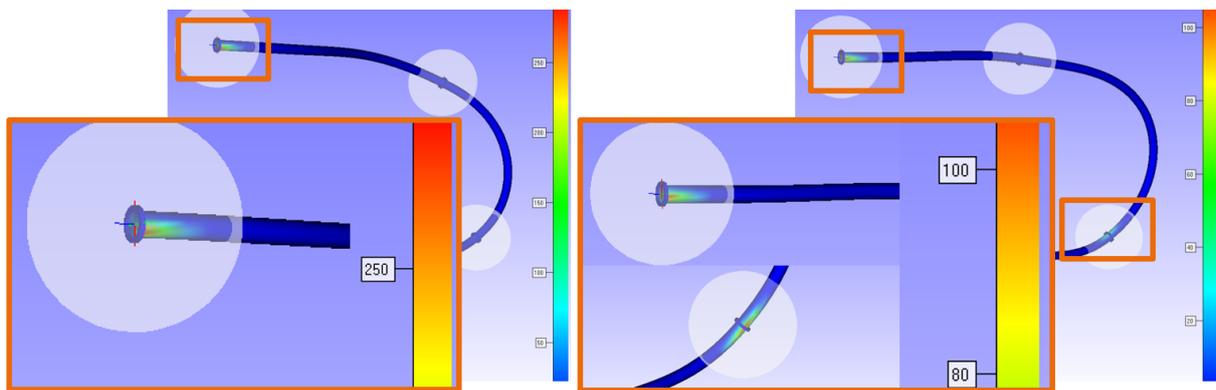
Figure 8: Results of a comparative LDA of two mounting variants. The right variant shows less damage and should be preferred.
