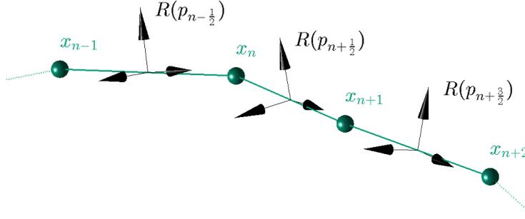
Figure 3: Staggered grid discretization of a geometrically exact Cosserat rod.
