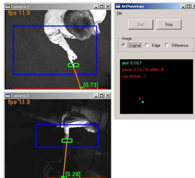
Figure 7: Screenshot of pointing tracking software showing the two (superimposed) camera images (top view, side view) and the application control window
