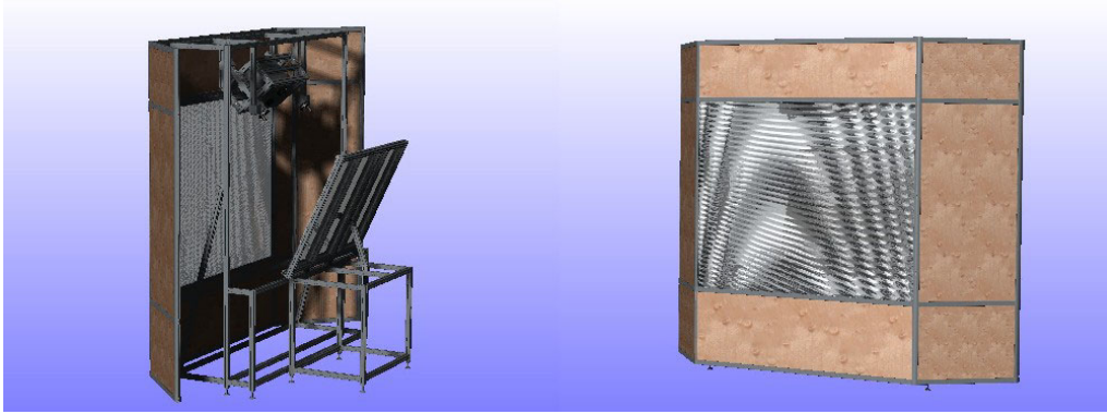
Figure 5: Sketch of projection canvas (back projection version)
