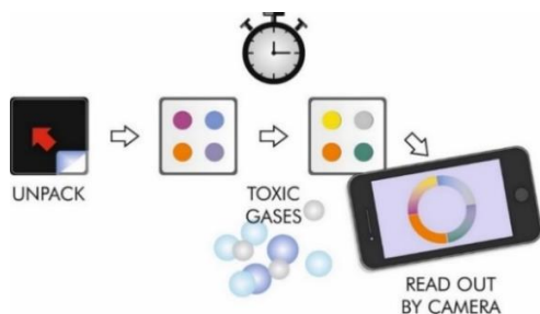
Fig. 1. Schematic illustration of the sensor principle. Colorimetric disposable sensor for the determination of toxic gases in the ambient air.
