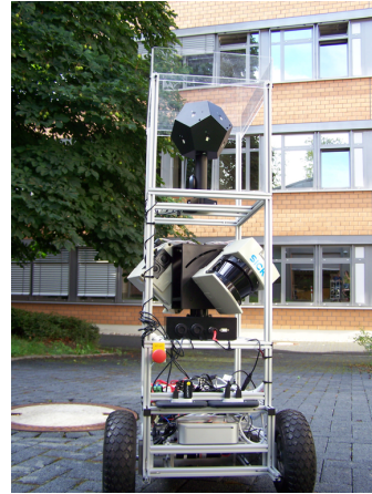
Fig. 9. Schematic survey of the evaluation platform DataBot . It is equipped with a panoramic vision system (sphere cube with 11 cameras), a continuous rotating 3D laser scanner, a GPS receiver, a landing platform for the quadrotor, batteries and control computers. A video can be seen at: http://de.youtube.com/watch?v=48WVz9cEir8
