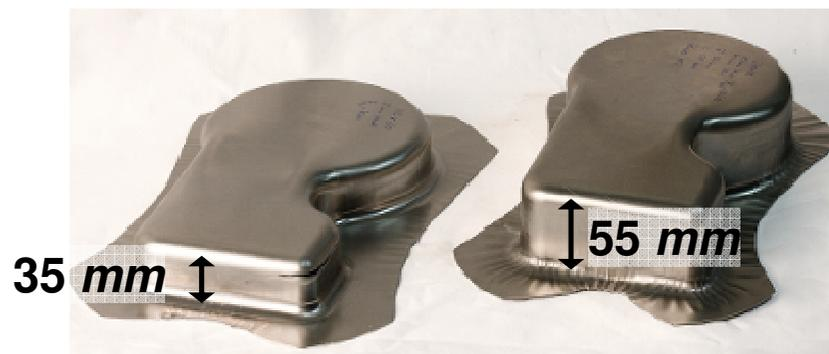
Schlüsselloch  $150 \text{ mm} \times 260 \text{ mm} \times 1 \text{ mm}$
