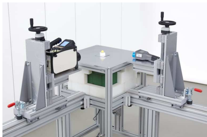
Figure 1: Setup of the static measurement system. Central cubic: in yellow: source, green: lead bricks, white: polyethylene bricks. Two guide rails with roller carriages with one detector each.
