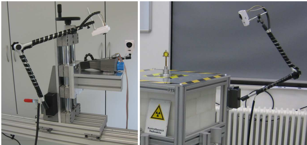
Figure 7: Video system. Left: roller carriage with camera observing the device display and clock and camera for the reference detector. Right: central cube with source observing camera towards the position of the extended source. The shown measurement device is a typical handheld device for illustration purpose.
