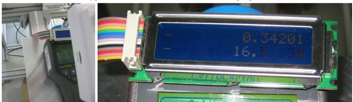
Figure 3: Display of the time measurement system in combination with a typical handheld device for illustration purpose. Left: display mounted on the detector filmed by the video camera (white box on the right). Right: LCD display upper line: previous measurement result (here: lift up time, 342 ms), lower line: actual measurement time; the last digit changes its position on the display on every update in order to compensate the slow LCD-refresh time. All times are given in seconds.
