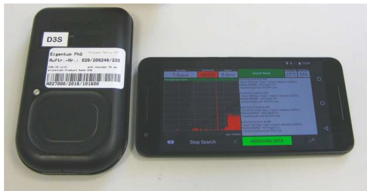
Figure 10: Test system D3S. Left: detector part, Right: smartphone with measurement running in search mode measuring a ^{226}\text{Ra} source. The left part shows the PCS significance over time, the right part the text box with status information, alerts, and measurement results.
