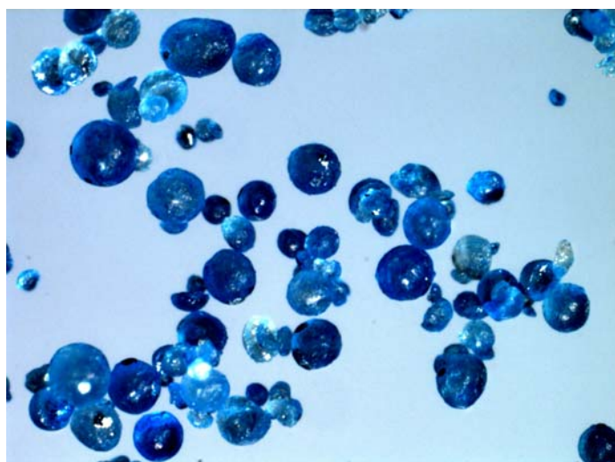
Figure 8: ADN-Prills coated with a polymer (from organic solvent)
