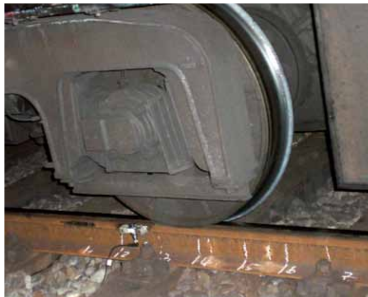
Acceleration sensor installed on the base of the track
