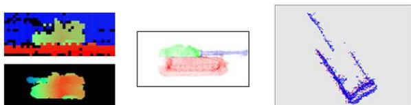
Figure 3. Range image matching: the expected range image (left, bottom) generated from the 3D model (centre) is matched with the range image (left, top). Point set matching: segmented on-target 3-D points (red, right) are matched with visible model points (blue, right), generated from the model.
