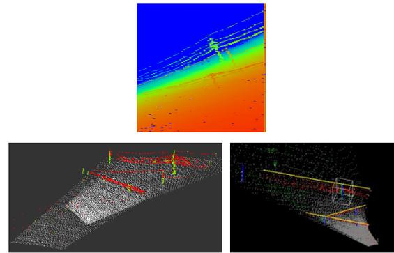
Figure 1. Range image processing for helicopter obstacle warning; top: laser radar image (color coded), below left: point cloud generation and classification, below right: recognition of masts and wires.
