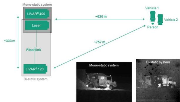
Figure 7. Bi-static configuration: shadow effect.
