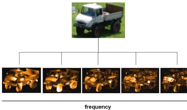
Figure 9. Visible image of a small truck and the 2d- vibration images at five different frequency bands - idling engine condition at different frequencies. Data were recorded using the 1.54  $\mu\text{m}$  - laser radar sensor with a resolution of 90 x 70 pixels at a range of 100 m.
