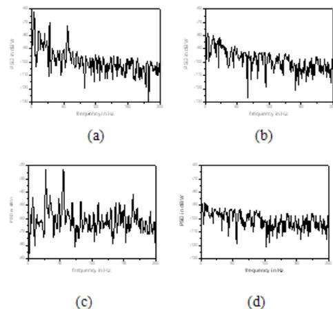
Figure 10. Off line-of-sight vibration measurements of a truck behind a wall. On wall: (a) engine on, (b) engine off. On target (as reference): (c) engine on, (d) engine off.
