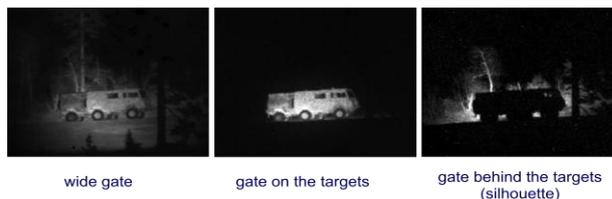
Figure 5. Different setting of the gate.
