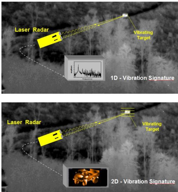
Figure 8. Measurement of 1D-and 2D-vibration signatures.
