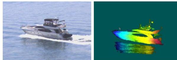
Figure 4. Visible and the color coded range profile image of a small boat, taken by the 3D flash laser system from ASC.
