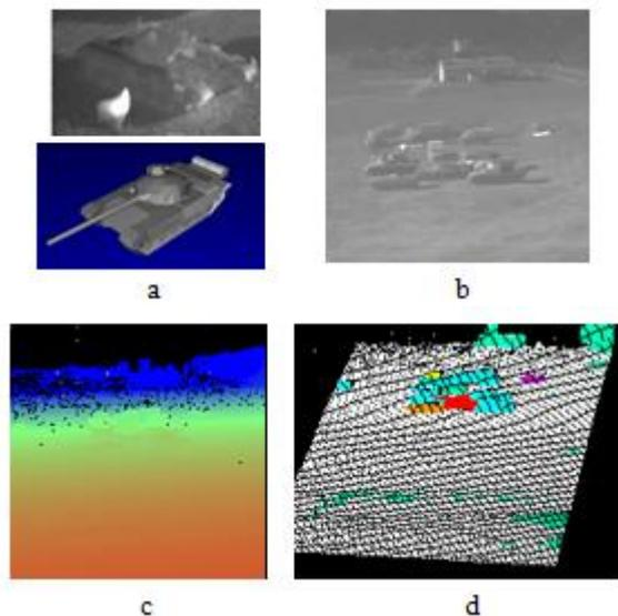
Figure 2. Comparison of object recognition in intensity vs. range data: the human observer fails to recognize model a in intensity image b, while automatic processing of the range image c correctly identifies the target (red in d). Human performance is not improved if an intensity model (a, top) is used.
