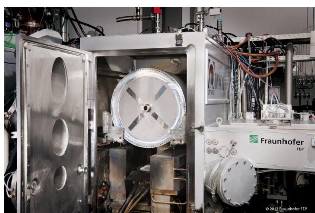
Figure 2: a) Brush cooling device, b) Gas cooling drum installed in FEP's in-line vacuum coating equipment for sheets and metal strips/foils "MAXI"
