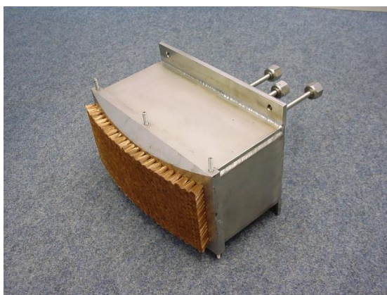
Figure 2: a) Brush cooling device, b) Gas cooling drum installed in FEP's in-line vacuum coating equipment for sheets and metal strips/foils "MAXI"
