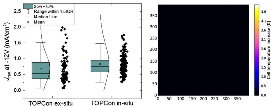
**Figure 10.** (Left) Reverse current density ( $J_{\text{rev}}$ ) measured by applying a reverse bias voltage of  $-12 \text{ V}$  for both ex situ and in situ routes; (right) infrared image of a representative TOPCon solar cell using thermography that shows no formation of hot-spots in the whole cell area.
