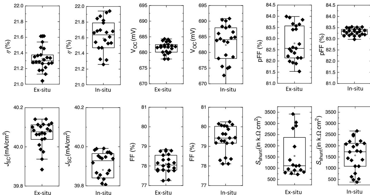
**Figure 9.** Current-voltage ( $I$ - $V$ ) results of the first-generation bifacial TOPCon cells ( $A_{\text{cell}} = 15.6 \times 15.6 \text{ cm}^2$ ) incorporating ADE poly-Si etching process for both ex situ (TOPCon\_ex situ) and in situ (TOPCon\_in situ) process routes.
