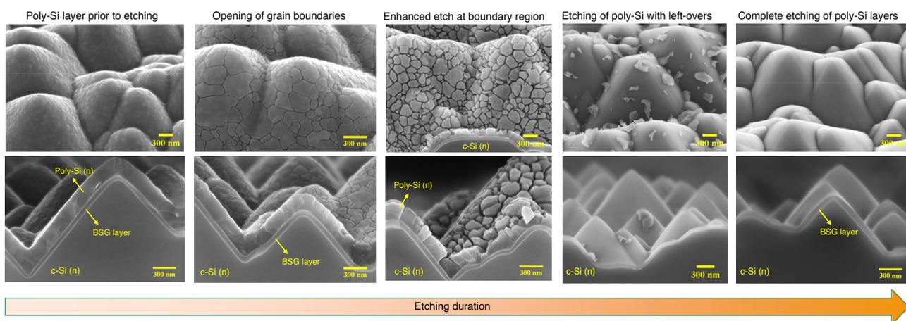
**Figure 4.** Tilted view (upper) and cross-sectional (lower) SEM images showing different phases of poly-Si etching after applying ADE process on n-doped polycrystalline silicon layers. Here, deposition of intrinsic a-Si layers is followed by ex situ doping in a POCl<sub>3</sub> tube furnace.
