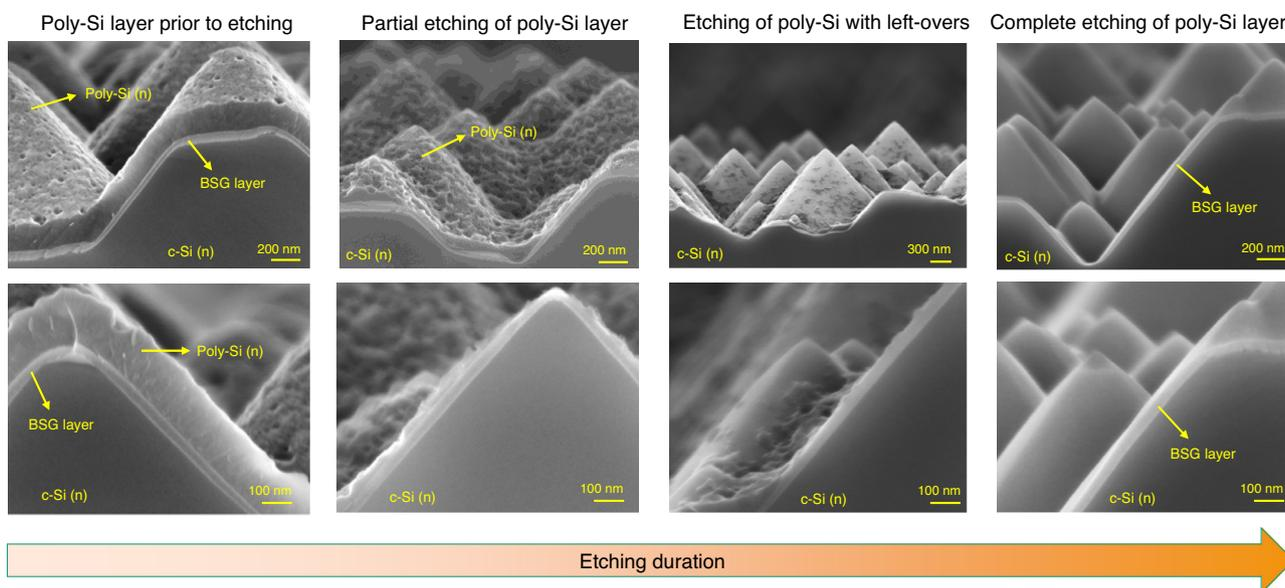
**Figure 5.** Tilted view (upper) and cross-sectional (lower) SEM images showing different phases of a/poly-Si etching after the exposure of in situ doped predominantly amorphous silicon layers to the F<sub>2</sub>/N<sub>2</sub> gas mixture. The samples are not annealed after LPCVD deposition process.
