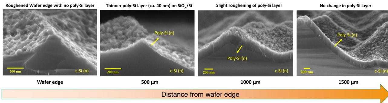
**Figure 7.** SEM images showing presence/absence of a-Si(n) layer for an increasing distance from the wafer-edge for the process D in Figure 6.
