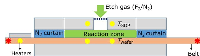
**Figure 1.** Schematic showing ADE tool used for the etching experiments. Here,  $T_{GDP}$  and  $T_{wafer}$  represent set-temperatures of the gas diffusion plate and Si wafer moving dynamically in a heated belt, respectively.
