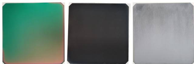
**Figure 8.** Photographs of solar cell precursors showing: (left) textured side after LPCVD deposition of a-Si(n) on top of BSG layer (left), (middle) textured side after ADE etching of a-Si(n) layer, and (right) rear side after ADE etching of a-Si(n) layer on the textured side.
