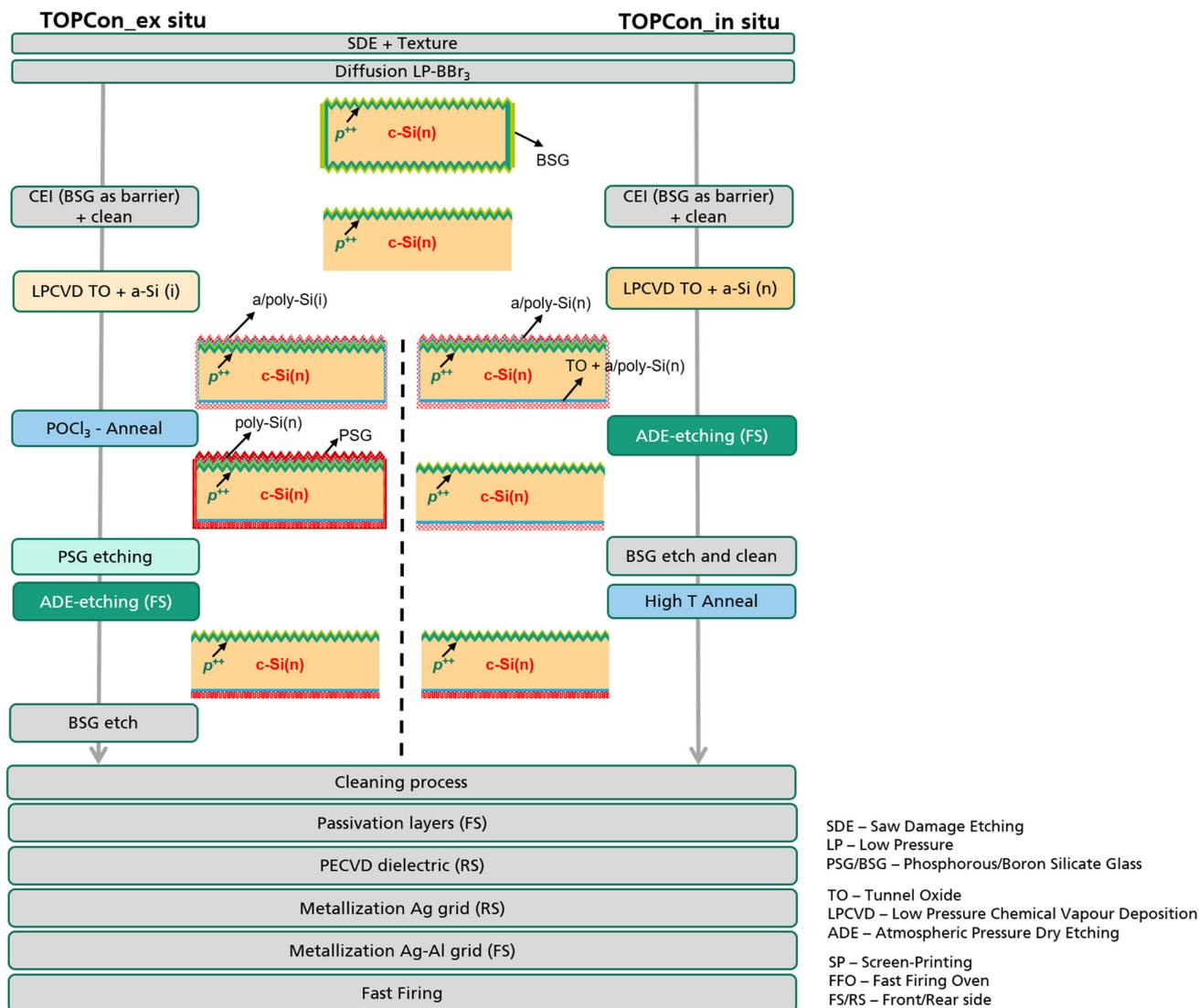
**Figure 3.** Process routes for both sides contacted n-TOPCon concepts using LPCVD polysilicon layers integrating ADE polysilicon etching process—TOPCon\_ex situ featuring deposition of intrinsic LPCVD layers followed by ex situ doping in  $\text{POCl}_3$  tube furnace, TOPCon\_in situ featuring in situ phosphorous-doped LPCVD layers.
