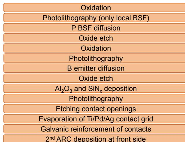
Fig. 8.12: Overview of the processing sequence for the fabrication of the bifacial solar cells.
