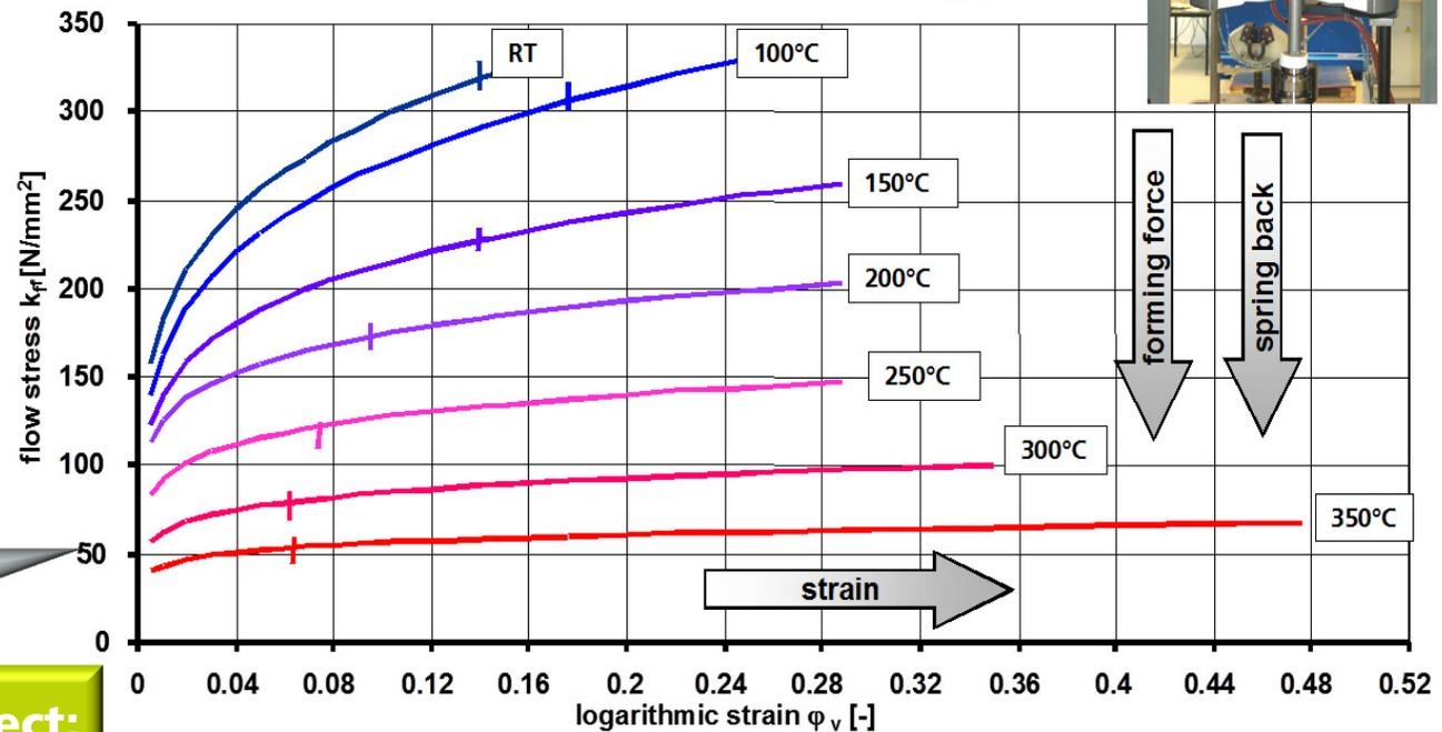
← → Tensile tests conducted regarding DIN EN10002-5
