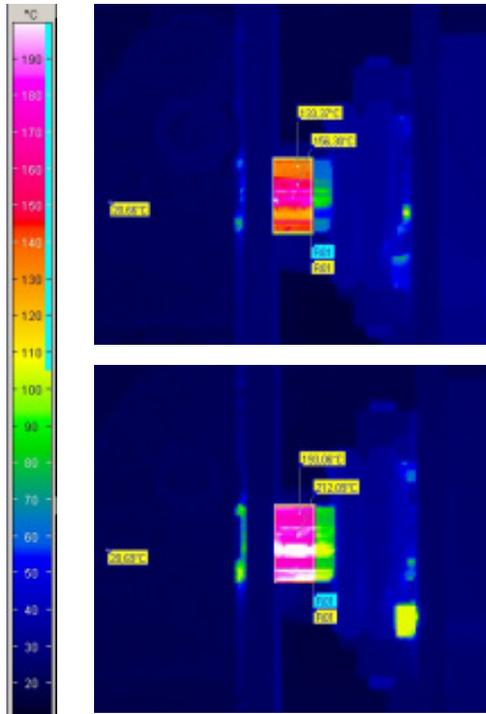
adjusting of power level for induction heating
