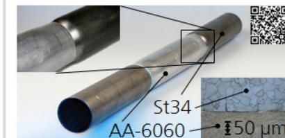
Magnetic pulse welded hybrid tube for hydroforming
