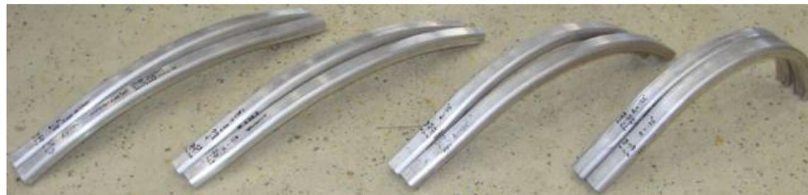
comparison of bended parts incl. and without induction heating
