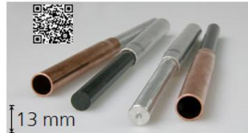
Multi material joints (Al, Cu, CFRP)
