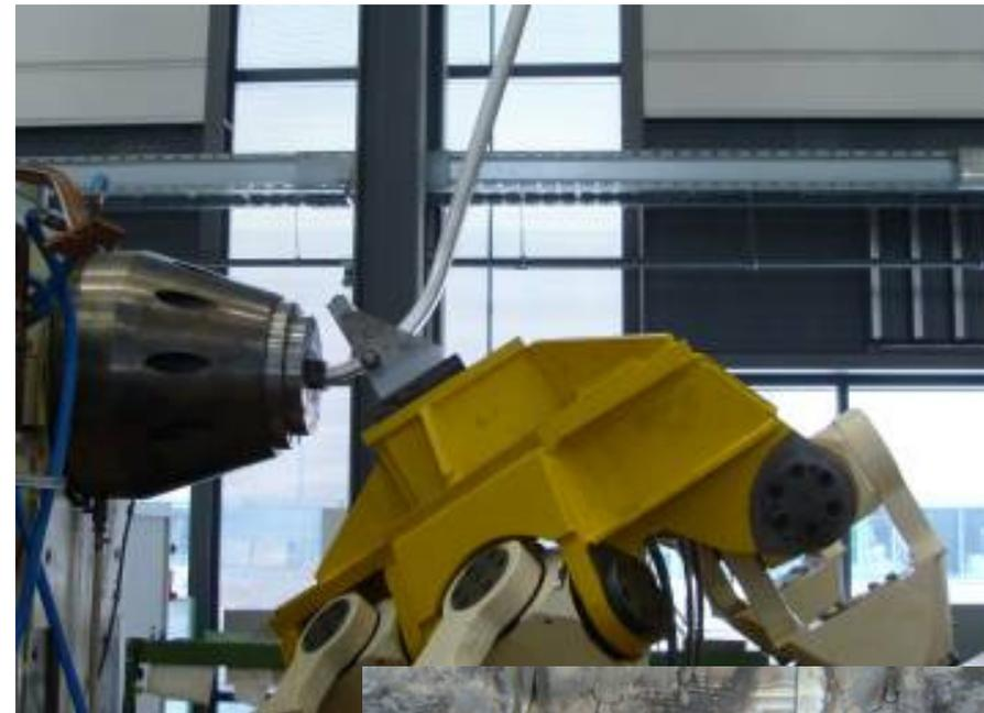
frame bending at parallel kinematic bending machine "HexaBend"
