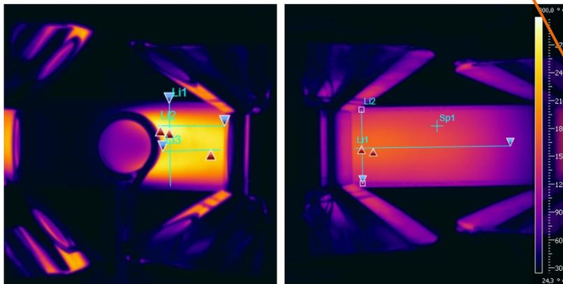
experimental determination of heat losses by radiation & roll contacts
