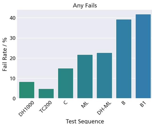
**FIGURE 7** Failure rate for different aging sequences. Criteria:  $P_{MPP}$  degradation, visual inspection, insulation, and wet leakage test
