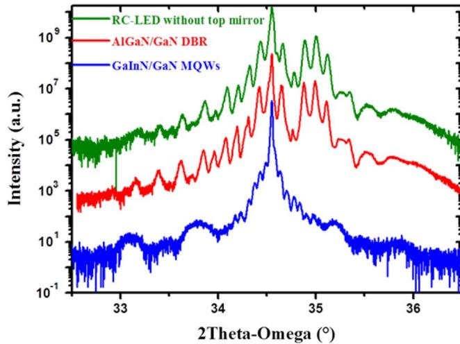
Fig. 2.  $2\theta - \omega$  scan around 002 reflection of RCLED without top mirror, AlGaN/GaN DBR and GaInN/GaN QW active region grown on GaN templates.
