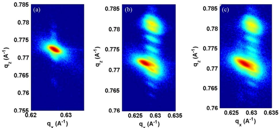
Fig. 3. RSM of the asymmetric 114 reflection of (a) InGaN/GaN MQWs grown on GaN template, (b) AlGaN/GaN DBR structure grown on GaN template and (c) RCLED without top mirror.
