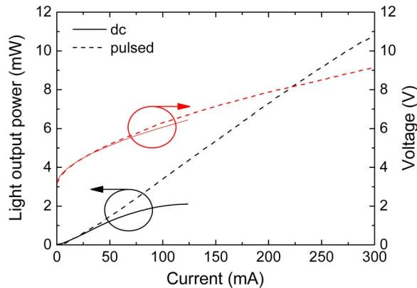
Fig. 8. Light output power current and voltage current characteristics from a  $200 \mu\text{m}$  diameter RCLED in dc and pulsed mode (pulse width  $1 \mu\text{s}$ , 0.1% duty cycle) at room temperature.
