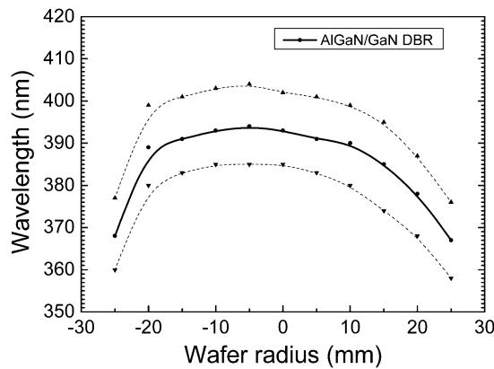
Fig. 5. Peak and half intensity wavelength of AlGaN/GaN DBR reflectance.
