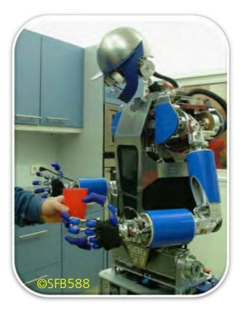
By the execution of a grasping task the robot has to cope with *internal* (kinematic) and *external* (surrounding, object) *uncertainties*
