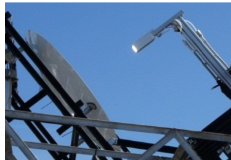
Figure 7: CPVT receiver and homogenizer assembled to the outdoor test setup at Fraunhofer ISE.
