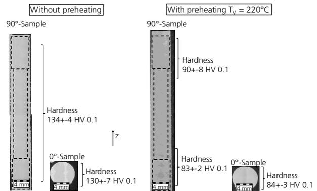
Figure 2: Cross section of samples for tensile tests, left: without preheating, right: with preheating ( $P_L = 960$  W)
