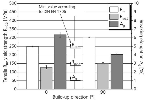
Figure 8: Mechanical properties for tensile specimens built with  $P_L = 960$  W,  $v_s > 1000$  mm/s and  $T_V = 220^\circ\text{C}$
