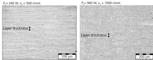
Figure 3: Microstructure of samples for tensile tests, left:  $P_L = 240$  W, right:  $P_L = 960$  W
