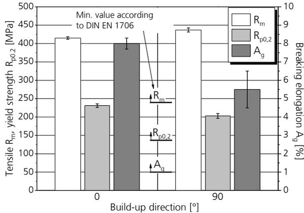
Figure 7: Mechanical properties for tensile specimens built with  $P_L = 960$  W,  $v_s > 1000$  mm/s
