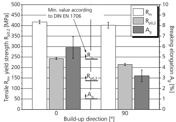
Figure 6: Mechanical properties for tensile specimens built with  $P_L = 240$  W,  $v_s = 500$  mm/s
