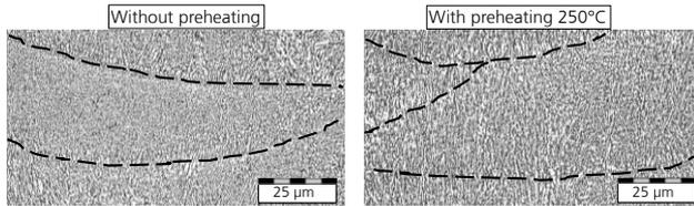
Figure 4: Microstructure of SLM samples built without (left) and with preheating (right)  $T_V = 250^\circ$  [15]
