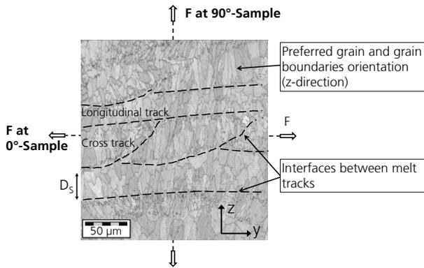
Figure 9: EBSD, Image Quality MAP of a SLM sample  $P_L = 240\text{ W}$ ,  $v_S = 500\text{ mm/s}$
