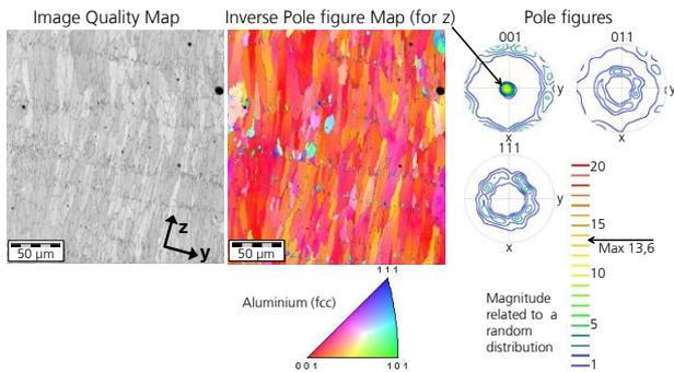
Figure 5: Exemplary EBSD results of one SLM sample ( $P_L = 960$  W)
