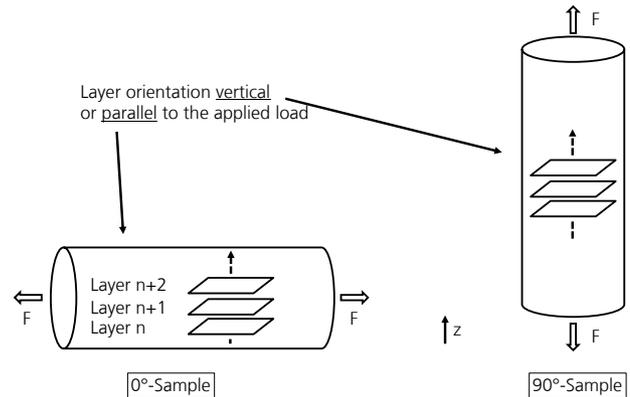
Figure 1: 0° and 90°-samples for tensile specimens, layer orientation depending on build-up direction (z)
