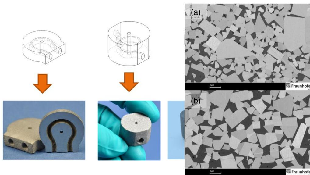
Figure 6: CAD- drawing of wire drawing dies with inner cooling channels and photos of sintered dies and microstructure of binder jet printed and sintered parts with 12 wt.% Co (a) and 17 wt.% Co (b)
