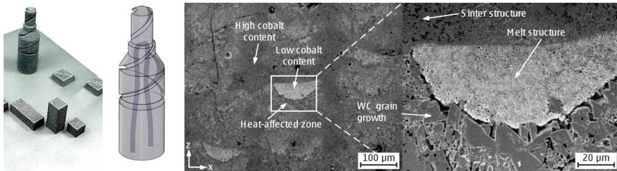
Figure 5: Overview, details and the microstructure of parts produced by SLS from Fraunhofer IPK [10]
