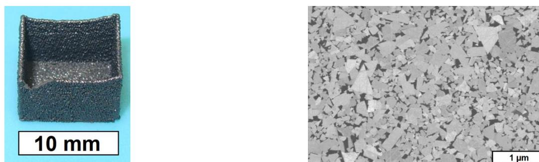
Figure 7: T3DP printed WC-10 Co test piece (left) and microstructure of sintered part (right) [19]
