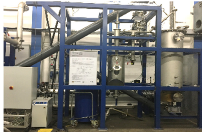
Updraft gasifier at UMSICHT (cheap, no tar)
