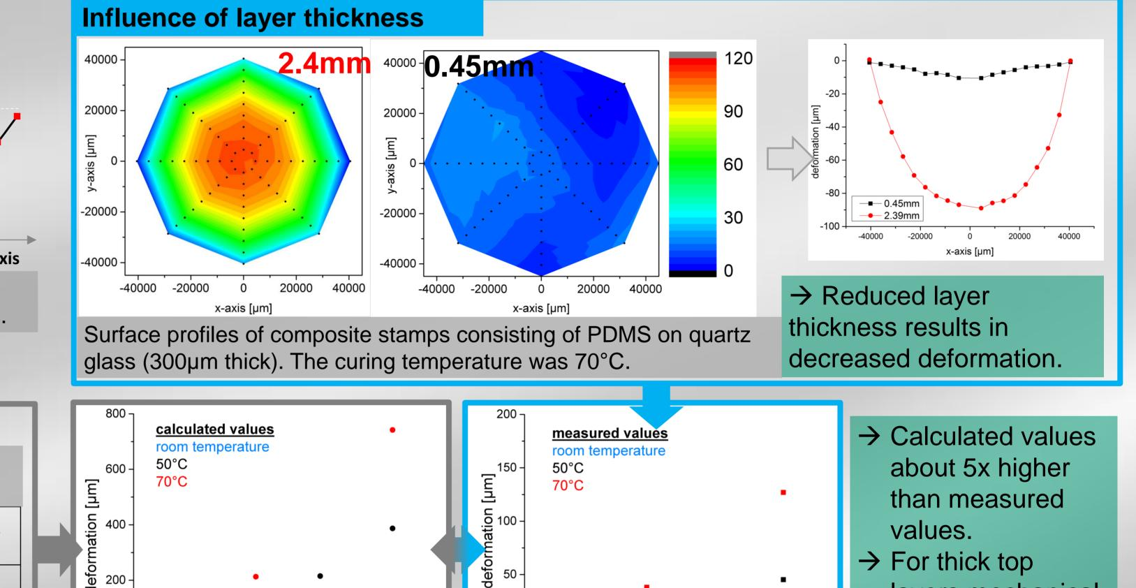
Deformation "w" calculated using trigonometric relations from the radius of curvature  $R_{c}$ .
