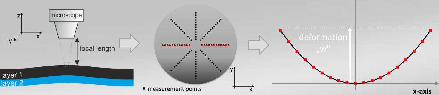
Substrate bottom side is measured to avoid influence of coating inhomogeneities. Reference measurements with a laser scanning flatness tester (Canon LSF-500) confirm the results.
