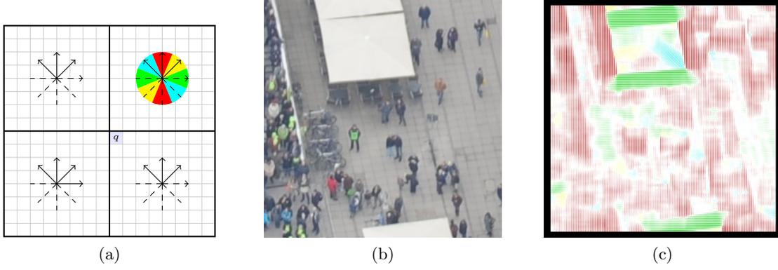
Figure 4. (a)  $16 \times 16$  neighborhood of a pixel  $q$  with the four subareas. The upper right subarea shows the colors used to indicate the different edge orientations. (b) Input image. (c) Colored illustration of the edge orientation feature  $\mathbf{f}_e$ . The color/pattern indicates the edge orientation  $f_{es,1}$ , the intensity indicates the strength  $f_{es,2}$ .
