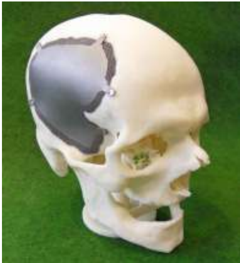
Figure 2: Patient-specific cranial-implant (Source: Fraunhofer Institute for Machine Tools and Forming Technology IWU, Chemnitz/Dresden)
