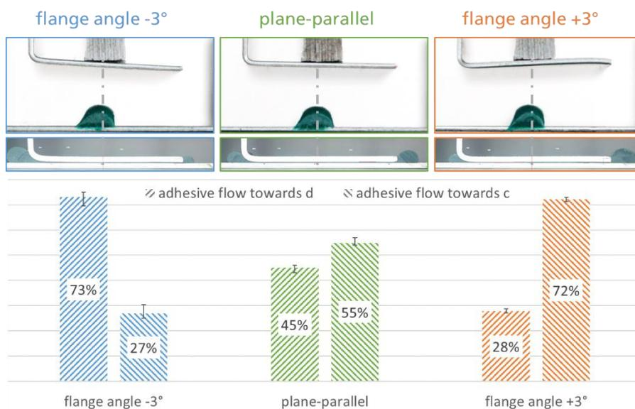
**Fig. 8.** Investigation of the adhesive flow direction with tilted inner part.
