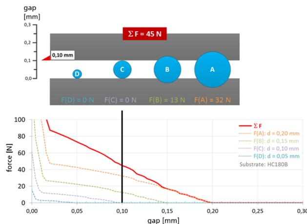
**Fig. 9.** Visualization of the glass bead calculation model.
