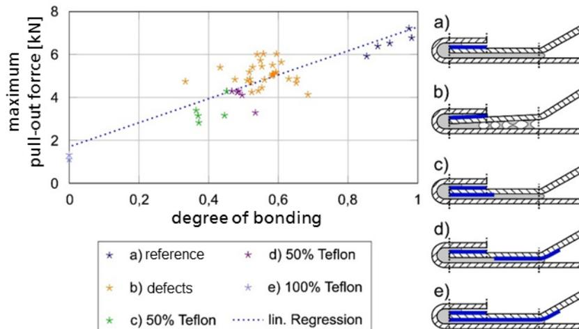
Fig. 12. Comparison of the pull-out forces as a function of the degree of bonding.
