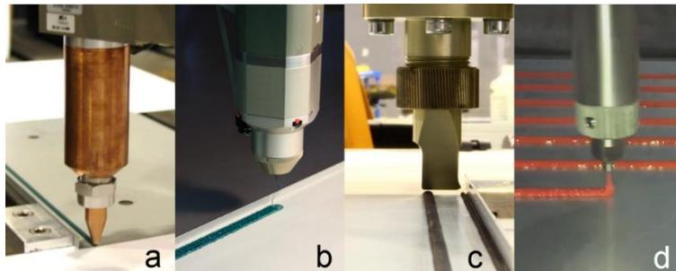
**Fig. 5.** Adhesive application: a) bead, b) Electric Swirl, c) double-bead, d) jet stream spraying [5].
