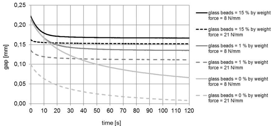
**Fig. 10.** Adhesive gap height with and without glass beads under constant load (amount of adhesive = 6.3 g/m, flange width inner part = 20 mm, nominal glass bead diameter = 0.2 mm, pressing speed = 0.1 mm/s)
