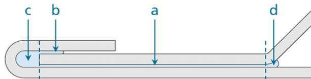
**Fig. 3.** Definition of the hem flange bonding areas [5].
