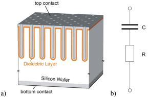
Fig. 1. a) Schematic device structure of the monolithic RC-snubber for power electronic applications, b) equivalent circuit
