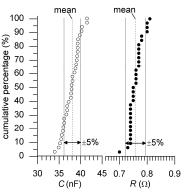
Fig. 3. Cumulative percentage of the capacitance and of the resistance for 33 RC-snubber with an area of 25 mm<sup>2</sup> over a 150 mm wafer
