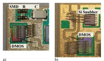
Fig. 7. Power hybrid with power switch and a) SMD snubber, b) monolithic silicon snubber
