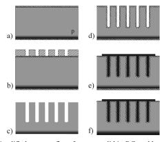
Fig. 2. Simplified process flow for a monolithic RC-snubber. a) thermal oxidation, back side doping and annealing, b) first lithography of the trenches, c) dry etching and removal of the photo resist and  $SiO_2$ , d) processing of the dielectric stack, e) processing and patterning the top electrode, f) cleaning of back side and processing the bottom electrode
