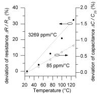
Fig. 4. Temperature dependent deviation of the capacitance ( $\Delta C$ ) and the resistance ( $\Delta R$ ) normalized to the values at 25°C ( $C_{25}$ ,  $R_{25}$ ), for temperatures between 25°C and 125°C
