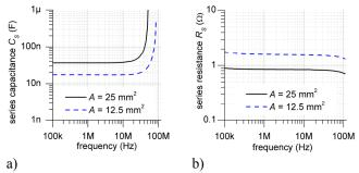
Fig. 6. a) Capacitance and b) resistance of diced RC-snubbers with a device area of 12.5  $\rm mm^2$  and 25  $\rm mm^2$  over a frequency range of 100 kHz to 110 MHz
