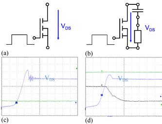
Fig. 8. MOS power switch a) without snubber, b) with RC snubber; simulated time dependent voltage during switching c) without snubber, d) with silicon chip snubber
