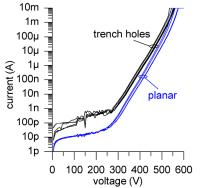
Fig. 5. I-V curves of planar and trench RC-snubbers with an device area of 1 mm<sup>2</sup>
