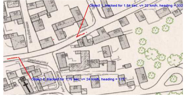
Figure 6. Two trucks have been detected and tracked on a UAV flight. Their velocities and headings can be computed, as in [23]
