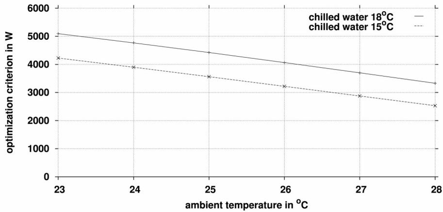
Figure 2 –Maximized optimization criterion at different ambient temperatures and for chilled water inlet temperatures of 15°C and 18°C
