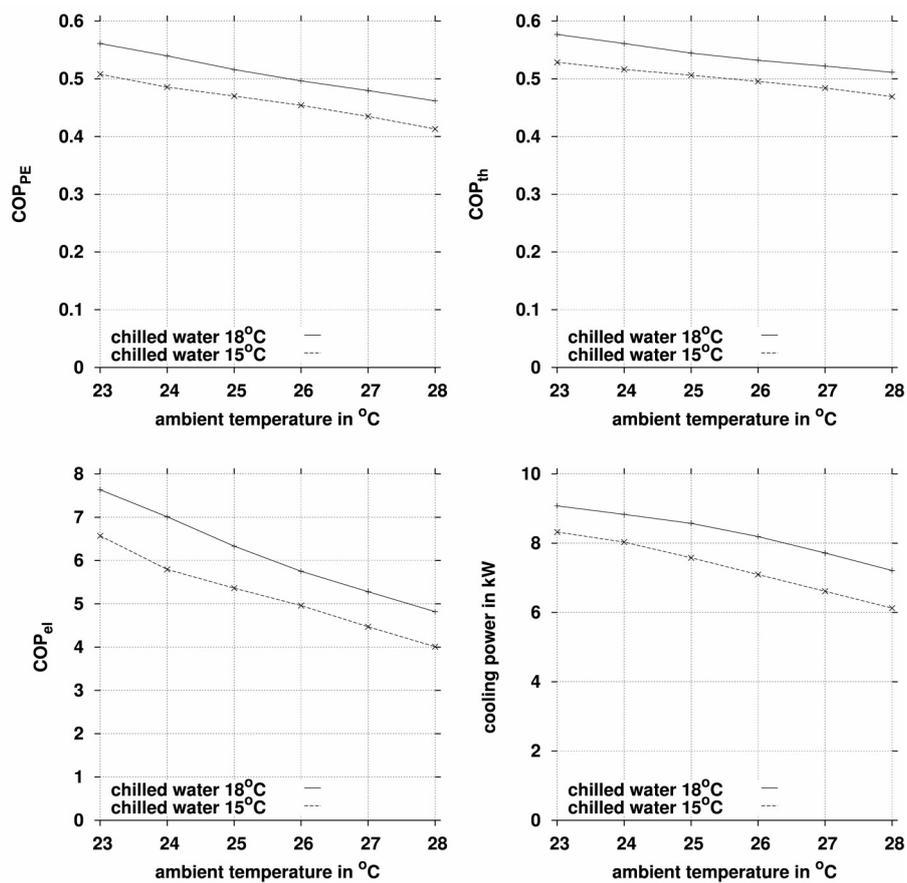
Figure 3 – Primary energy efficiency ( $COP_{PE}$ ), thermal  $COP_{th}$ , electrical  $COP_{el}$  and the cooling power of the TDCs
