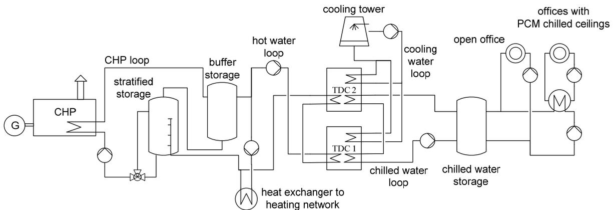
Figure 1 – Hydraulic scheme of the CHCP system.
