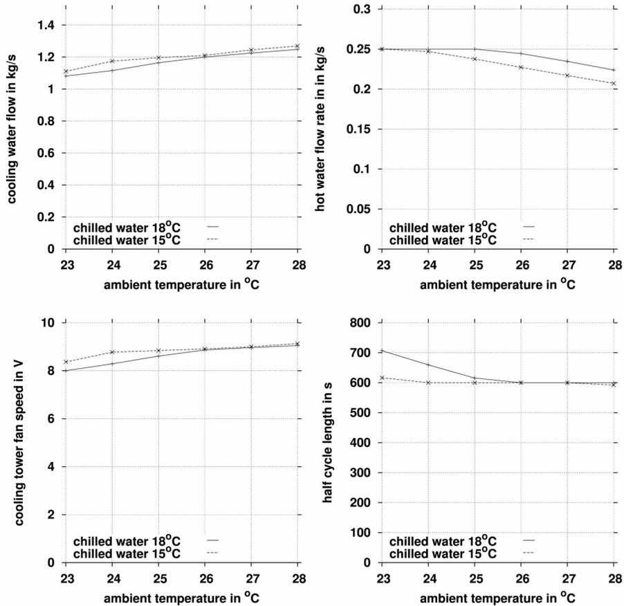
Figure 4 –Control strategy for the hot water and cooling water pump as well as the cooling tower fan signal and the half cycle length of the TDC for different ambient temperatures and chilled water inlet temperatures.
