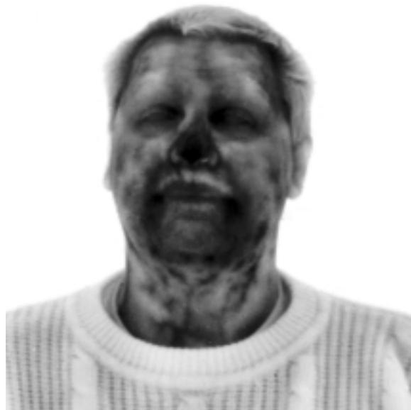
Fig. 2: Thermal image of an AIM colleague taken with the 256x256 InAs/GaSb SL camera. Brighter areas indicate colder parts.
