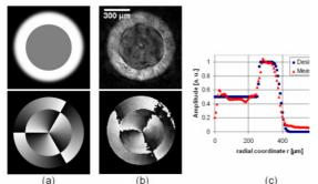
Fig. 4: CGH with two regions of different non-zero amplitude and changing spiral phase pattern with opposite sense of rotation. (a) Desired amplitude and phase. (b) Measured amplitude and phase using lensless digital holography. (c) Radial amplitude profile of the measured and desired amplitude (in arbitrary units).
