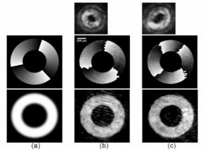
Fig. 3: CGHs with circular amplitude and spiral phase. (a) desired phase (top) and amplitude (bottom); (b) interferogram 140 mm behind CGH (spiral phase from 0 to 6  $\pi$ ) with tilted reference beam (top), reconstructed phase and amplitude in the plane of the CGH (scale bar is 200  $\mu$ m); (c) interferogram (top), reconstructed phase and amplitude for CGH with a circular amplitude and spiral phase ranging from 0 to  $8\pi$
