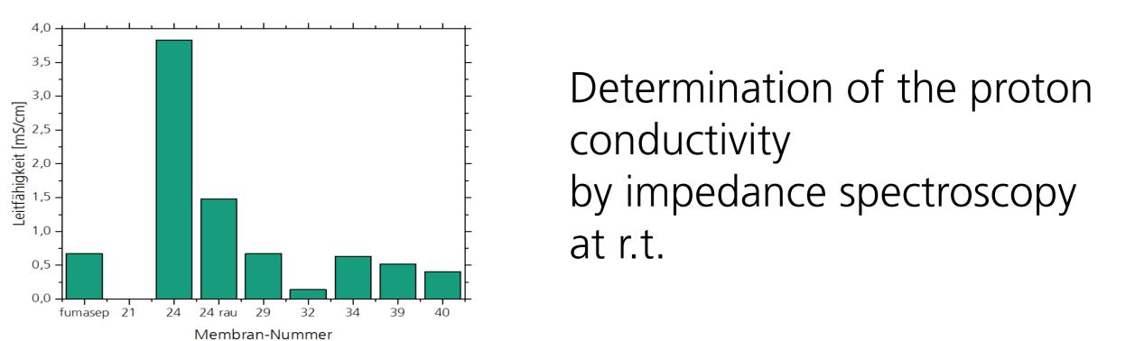
Proton conductivity comparable or higher as Nafion<sup>®</sup> membrane
