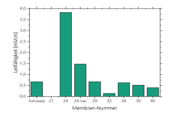
Determination of the proton conductivity by impedance spectroscopy at r.t.
