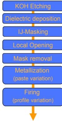
**Figure 2:** The process flow shows the processing steps.
