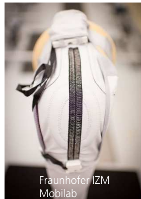
Knee brace – Angle measurement
