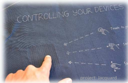
Jacquard weaved touch control panel (Google, TE Connectivity)
