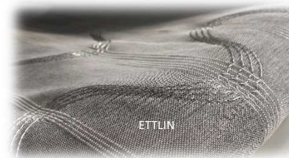
Leno weaved circuit (Conductors can be integrated in curved designs)
