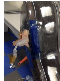
Epoxy injection under vacuum
