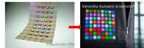
Textile display: Smart Pixel bonded onto Jaquard woven fabric
