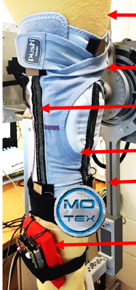
Artificial knee test bench
