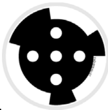
Fig. 5. The coded MCT-MXT marker
