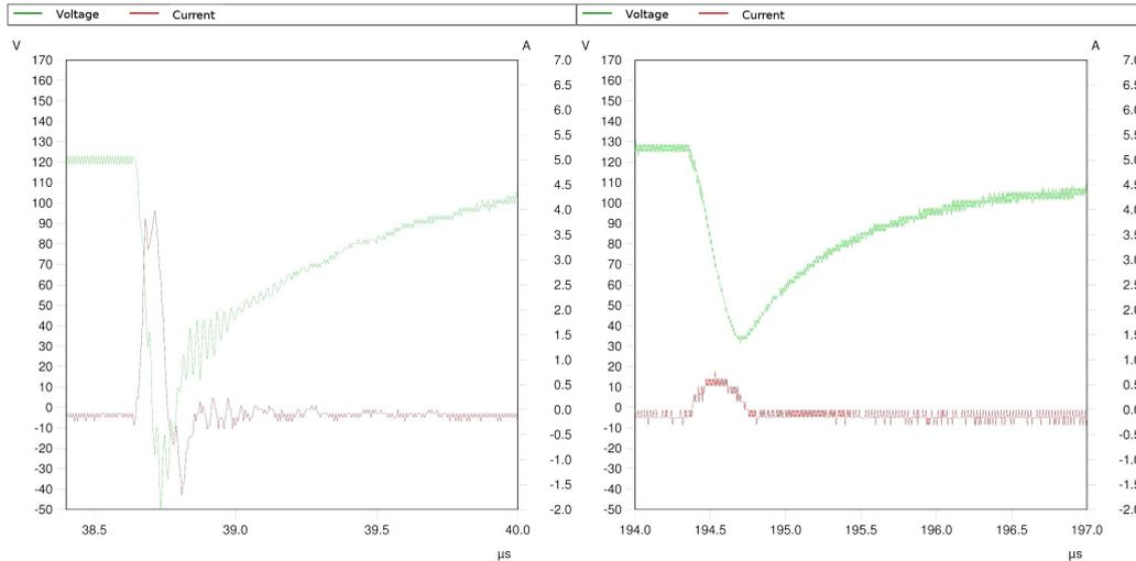
**FIGURE 4.** Discharge signal a) metal micro-EDM b) micro-EDM of starting layer in ceramic
