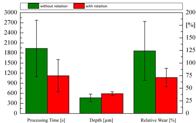
**FIGURE 3.** Machining results with and without electrode rotation: processing time [s], bore depth [ $\mu m$ ], wear [%] ( $Y_2O_3-ZrO_2$ )
