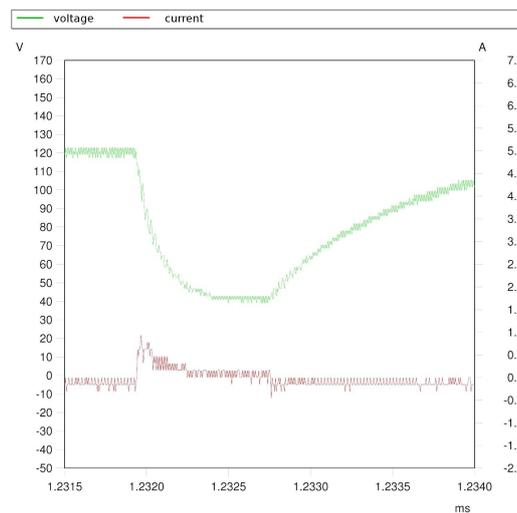
**FIGURE 5.** current and voltage signal of *ceramic* discharge in micro-EDM (base material stage)
