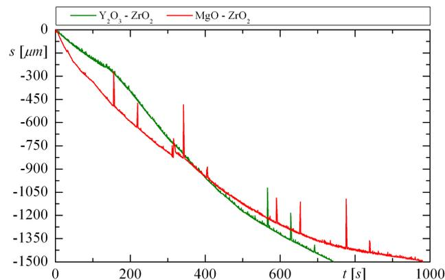
**FIGURE 6.** Process speed of micro-EDM in Y<sub>2</sub>O<sub>3</sub> and MgO stabilized ZrO<sub>2</sub> ceramic. Peaks in the graph represent short retracting movements of the tool electrode.
