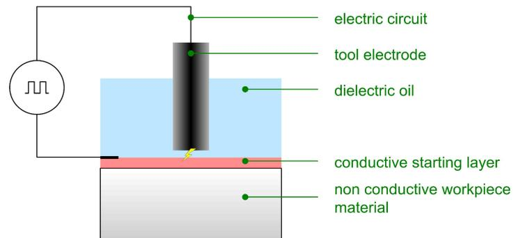
**FIGURE 2.** Assisting electrode setup
