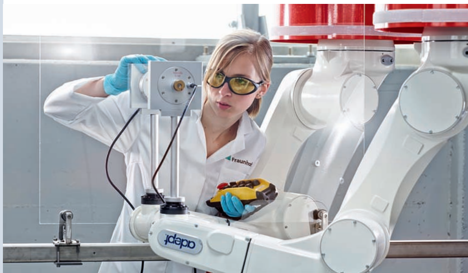
Air-coupled ultrasound: an industrial robot linked to the ultrasound testing system scans the component. © Uwe Bellhäuser
