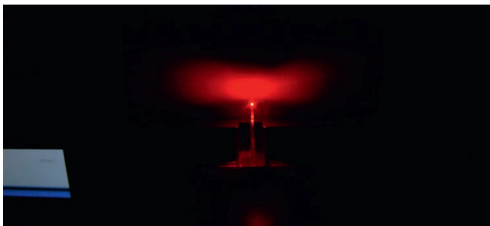
Example of radial emission from a laser-structured fiber tip with an internal cone. © Fraunhofer IZM
