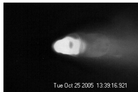
CMOS Image: Root Fusion with Key Hole
