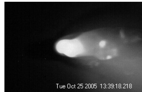
CMOS Image: Weld Spatter
