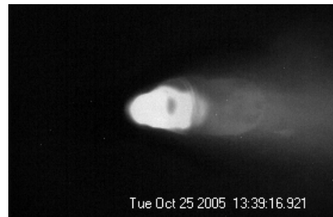
CMOS Image: Root Fusion with Key Hole
