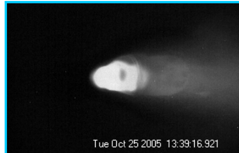
CMOS Image: Root Fusion with Key Hole
