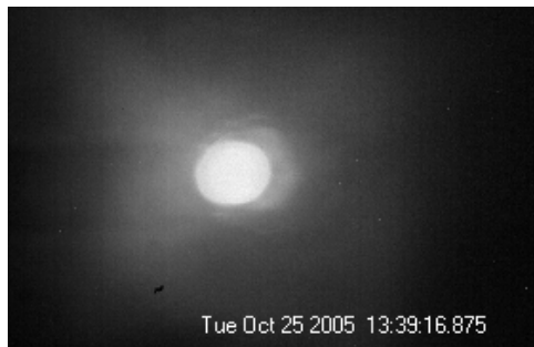
CMOS Image: Start without Root Fusion
