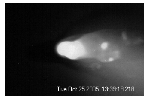
CMOS Image: Weld Spatter
