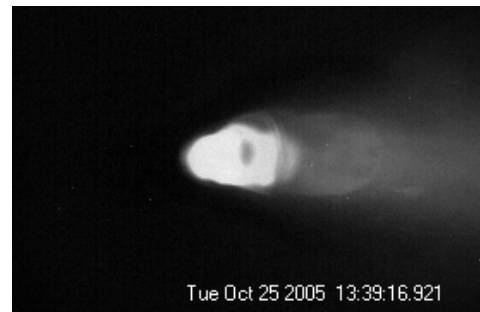
CMOS Image: Root Fusion with Key Hole
