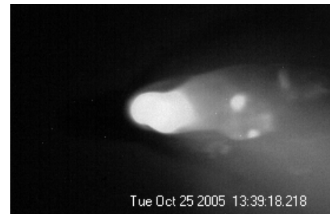
CMOS Image: Weld Spatter
