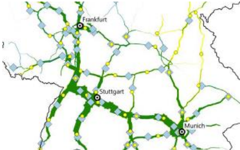
Figure 2: Optimal allocated fast charging stations along the highway around Stuttgart (own simulation)
