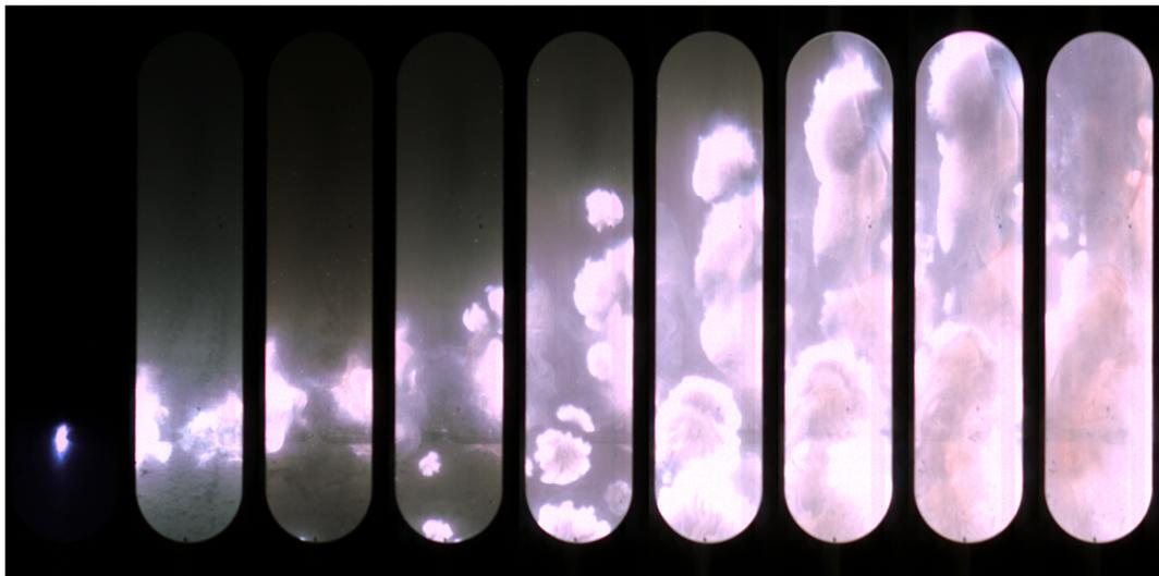
**Figure 5: Series of aluminum particles combustion in the modified Hartmann-Apparatus.**
