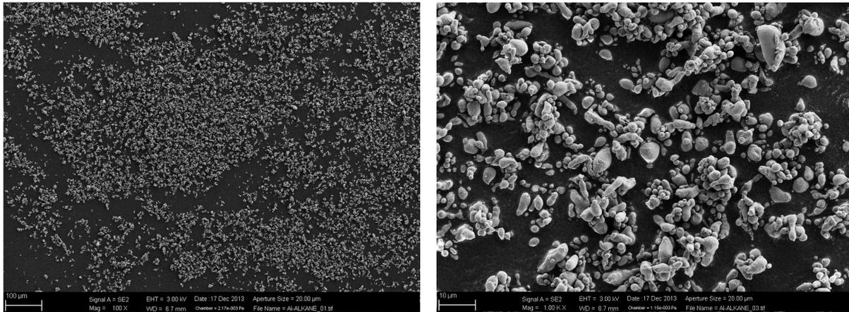
**Figure 3: SEM micrographs of aluminum particles (Sibthermochim,  $d_{0.5}=4,25 \mu\text{m}$ ; SEM magnification: 100x and 1000x).**
