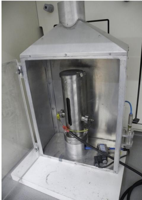
**Figure 2: Picture of the modified Hartmann-Apparatus at the Fraunhofer ICT.**
