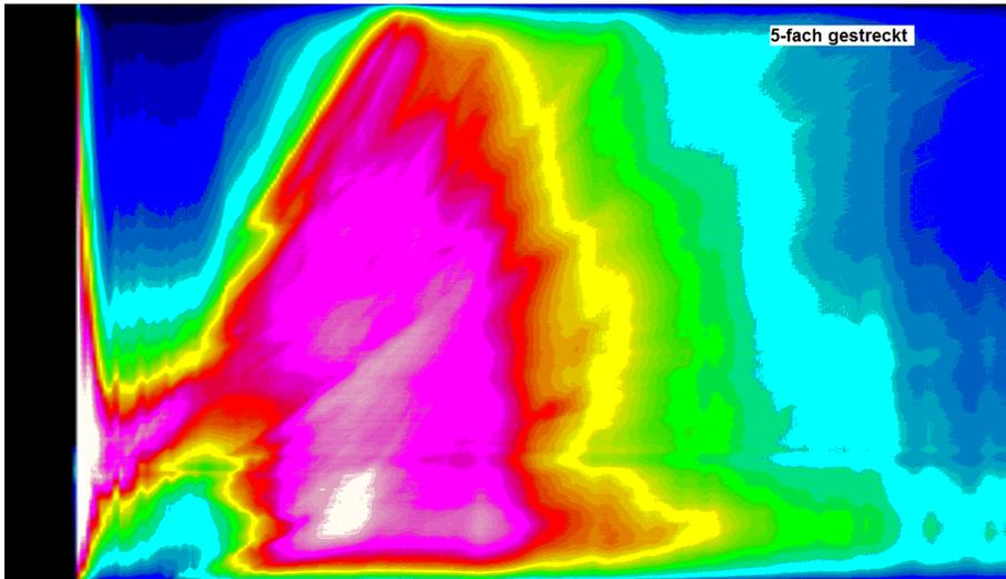
Figure 7: Evaluation of the brightness distribution of the single images in the case of aluminum particles (500 g/cm³).
