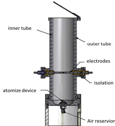
**Figure 1: Schematic design of the modified Hartmann-Apparatus.**
