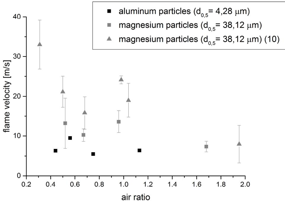
**Figure 9: Flame propagation velocity dependent of air ratio (black: aluminum particles; grey: magnesium particles; triangles already published in (1)).**
