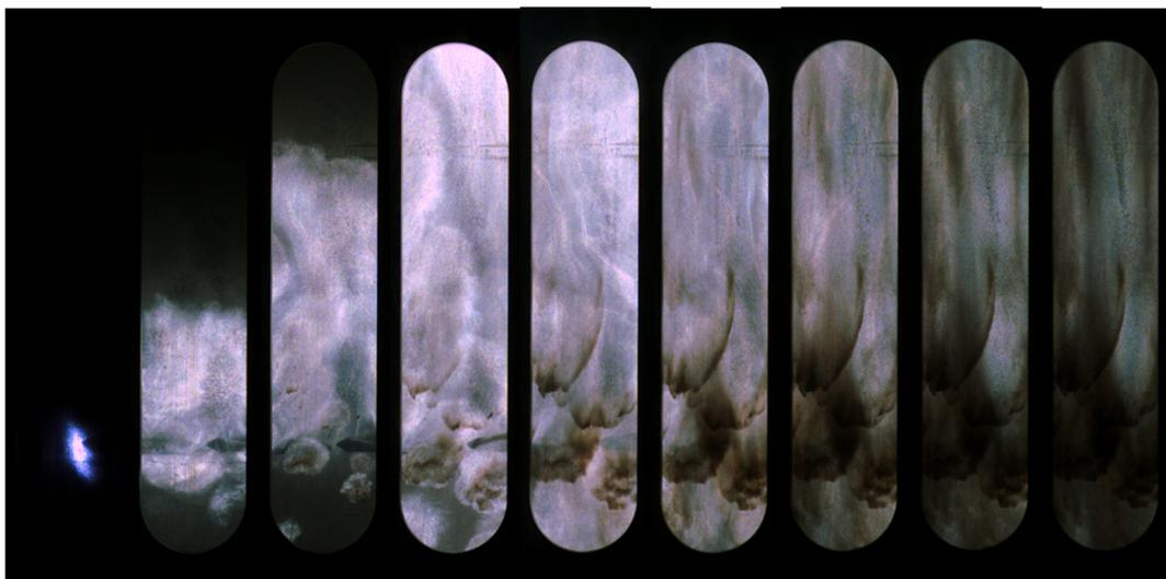
**Figure 6: Series of magnesium particles combustion in the modified Hartmann-Apparatus.**
