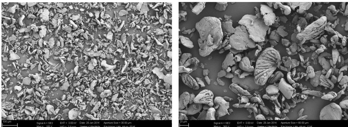
**Figure 4: SEM micrographs of magnesium particles (Alfa Aesar,  $d(0.5) = 38.120 \mu\text{m}$ ; SEM magnification: 100x and 300x).**
