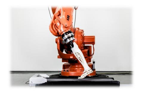
Simulate human gait on an industrial robot
