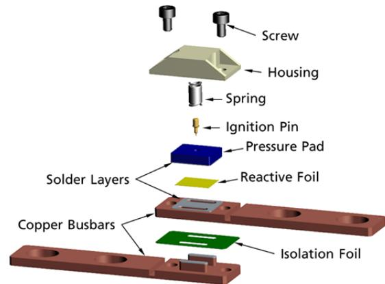
Fig. 4. Exploded view of the assembly of a high-current low-voltage power antifuse bypass device prototype.
