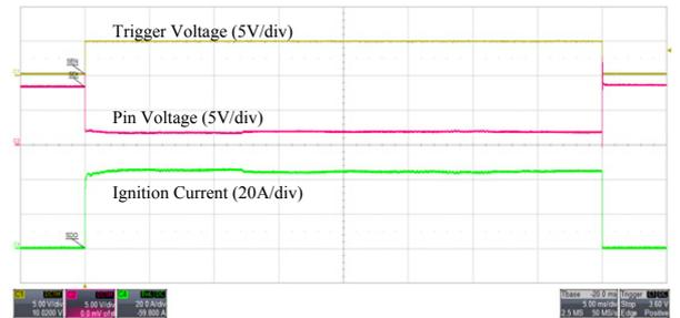
Fig. 13. Oscillogram of the reactive foil ignition sequence.
