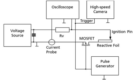
Fig. 12. Schematic of the measurement setup used to ignite the antifuses and measure the ignition delay and the reaction period.
