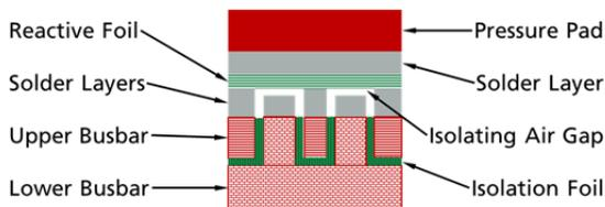
Fig. 7. Cross-section AA' of the assembly of a high-current low-voltage antifuse device as shown in Fig. 5.
