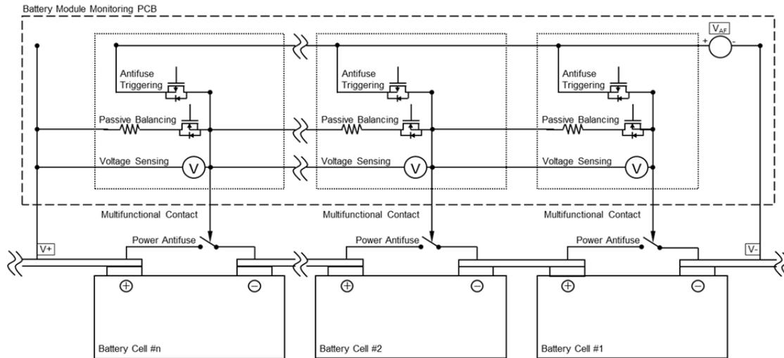
Fig. 10. Schematic of a battery module showing the general principle of series connected battery cells having an integrated antifuse and a multifunctional contact allowing the three following functions over a single wire: cell voltage sensing, passive balancing (i.e., charge equalization), and antifuse ignition.
