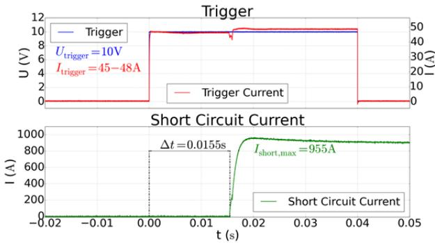
Fig. 15. Short circuit current when shorting a 30 Ah prismatic high-power lithium-ion LFP/Graphite battery cell charged at 100% SOC.
