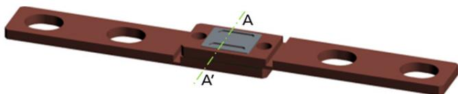
Fig. 5. Assembly of a high-current low-voltage antifuse device showing the difference in height ensuring the electrical isolation in the pristine state. The cross-section AA' is shown in Fig. 7.
