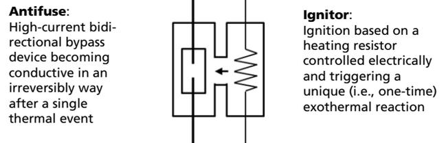
Fig. 3. Proposed electrical symbol for the new controlled power antifuse device in which the antifuse device symbol is shown directly associated to the electro-thermal ignitor device symbol.
