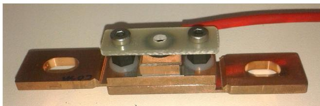
Fig. 6. Photography of a power antifuse device with its trigger contact.
