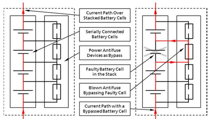
Fig. 1. Battery system consisting of battery cells connected in series and having integrated antifuses. The current path is shown during normal operation on the left side and in case a battery cell has failed and the current must be bypassed by one of the antifuses on the right side.
