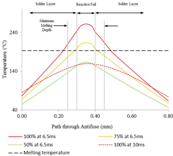
Fig. 11. Thermal simulation results obtained with an ambient temperature of  $22^\circ\text{C}$  and a reaction period of 6.5 ms. The temperature profile for various remaining energies in the reactive foil is plotted. The minimum melting depth for activation corresponds to the equivalent height difference shown in Fig. 7 by the isolating air gap. No thermal barrier was considered between the pressure pad and the busbars.
