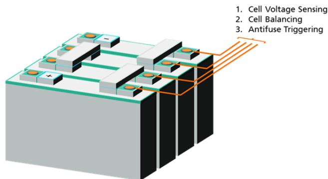
Fig. 9. Assembly of battery cells in a battery module showing the connection to a multifunctional battery cell contact allowing all three functions over a single electrical cable connection: cell voltage sensing, cell balancing (i.e., charge equalization), and antifuse triggering.
