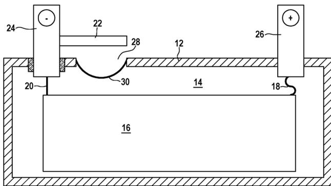
Fig. 2. State-of-the-art 60 Ah prismatic lithium-ion battery cell (14) providing an integrated pressure sensitive safety device (28) [8] [9]. In contrary to the antifuse, the device (28) cannot be triggered by an external signal and is therefore not able to provide a controlled irreversible shutdown of the battery cells in case of a vehicle crash.
