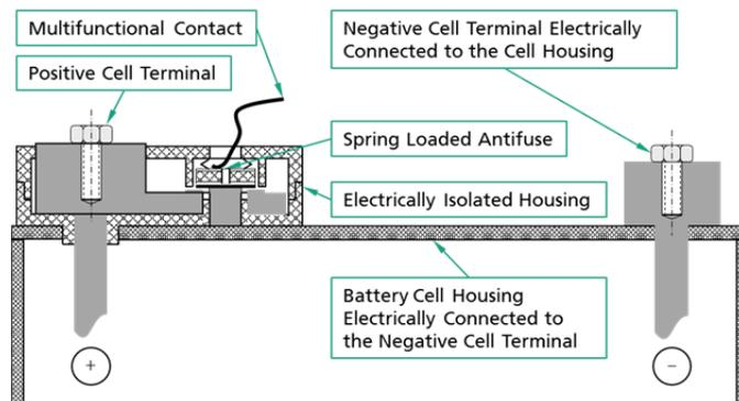
Fig. 8. Prismatic hard-case battery cell drawing showing the integrated power antifuse and its multifunctional electrical contact for cell voltage sensing, cell balancing and antifuse triggering.
