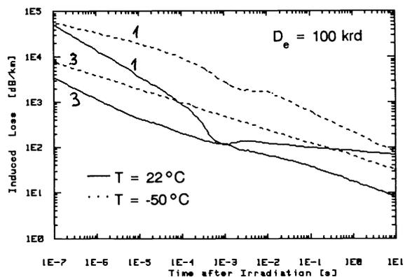
Figure 16: Change of the induced loss after pulsed irradiation with temperature. 1: Fibre Philips SM FL 1048C,  $\lambda = 1309$  nm,  $P = 20$   $\mu$ W; 3: Fibre Heraeus SS 1.2 152/90,  $\lambda = 840$  nm,  $P = 10$   $\mu$ W.
