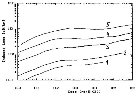
Figure 12: Induced loss as a function of dose for five different dose rates.  $\lambda = 865$  nm,  $P = 10 \mu\text{W}$ ,  $T = 22^\circ\text{C}$ .  $\dot{D} = 0.25$  rd/s (1),  $1$  rd/s (2),  $4.6$  rd/s (3),  $20.4$  rd/s (4), and  $162$  rd/s (5).
