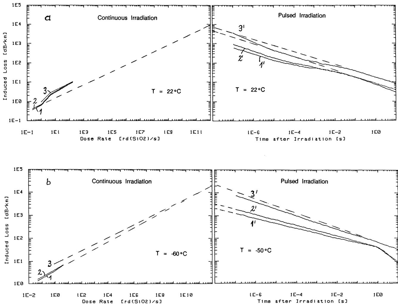
Figures 14a,b: Comparison of continuous and pulsed irradiation.  $D = 3 \cdot 10^3$  rd (1,1'),  $10^4$  rd (2,2'), and  $10^5$  rd (3,3'). Corresponding dose rates of the pulsed irradiations:  $\dot{D}_e = 10^{11}$  rd/s (1'),  $3 \cdot 10^{11}$  rd/s (2'), and  $3 \cdot 10^{12}$  rd/s (3').
