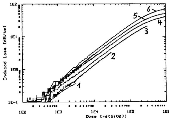
Figure 1: Induced loss as a function of dose for six different dose rates.  $\lambda = 1309$  nm,  $P = 20$   $\mu\text{W}$ ,  $T = 22^\circ\text{C}$ .  $\dot{D} = 0.05$  rd/s (1),  $0.25$  rd/s (2),  $1$  rd/s (3),  $4.4$  rd/s (4),  $19.8$  rd/s (5), and  $161$  rd/s (6).
