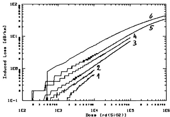
**Figure 6:** Induced loss as a function of dose for six different dose rates.  $\lambda = 1308 \text{ nm}$ ,  $P \approx 10 \text{ } \mu\text{W}$ ,  $T = 22^\circ\text{C}$ .  $\dot{D} = 0.05 \text{ rd/s}$  (1),  $0.25 \text{ rd/s}$  (2),  $1^7 \text{ rd/s}$  (3),  $5 \text{ rd/s}$  (4),  $21.7 \text{ rd/s}$  (5), and  $189 \text{ rd/s}$  (6).
