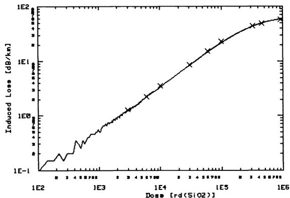
Figure 17: Comparison of the induced losses during continuous irradiation measured by conventional transmission loss measurement (—) and OTDR (xxx). Fibre: Philips SM SA 4015C;  $\dot{D} = 1200$  rd/min,  $\lambda \approx 1300$  nm,  $P \approx 0.1$   $\mu$ W,  $T = 22^\circ$ C.
