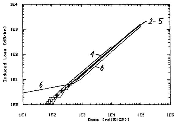
**Figure 9:** Induced loss as a function of dose for six different dose rates.  $\lambda = 1308 \text{ nm}$ ,  $P \approx 10 \text{ } \mu\text{W}$ ,  $T = 22^\circ\text{C}$ .
