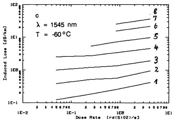
Figures 2a-c: Induced loss as a function of dose rate;  $P = 20 \mu\text{W}$ .
