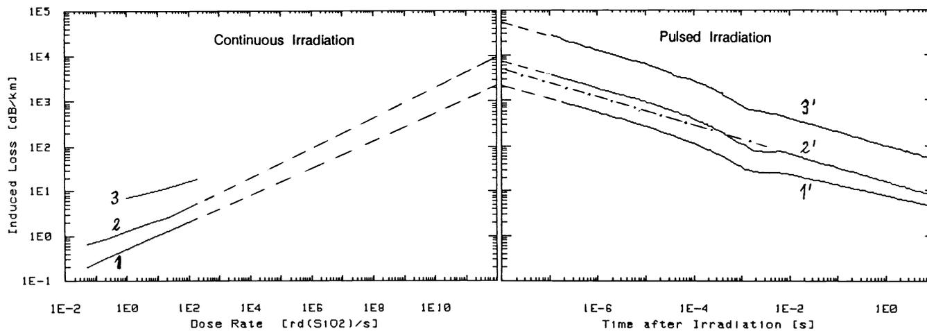
**Figure 8:** Comparison of continuous and pulsed irradiation.  $\lambda = 1308 \text{ nm}$ ,  $P \approx 10 \text{ } \mu\text{W}$ ,  $T = 22^\circ\text{C}$ .  $D = 3 \cdot 10^3 \text{ rd}$  (1,1'),  $10^4 \text{ rd}$  (2,2'), and  $10^5 \text{ rd}$  (3,3'). Corresponding dose rates of the pulsed irradiations:  $\dot{D}_e = 10^{11} \text{ rd/s}$  (1'),  $3 \cdot 10^{11} \text{ rd/s}$  (2'), and  $3 \cdot 10^{12} \text{ rd/s}$  (3').
