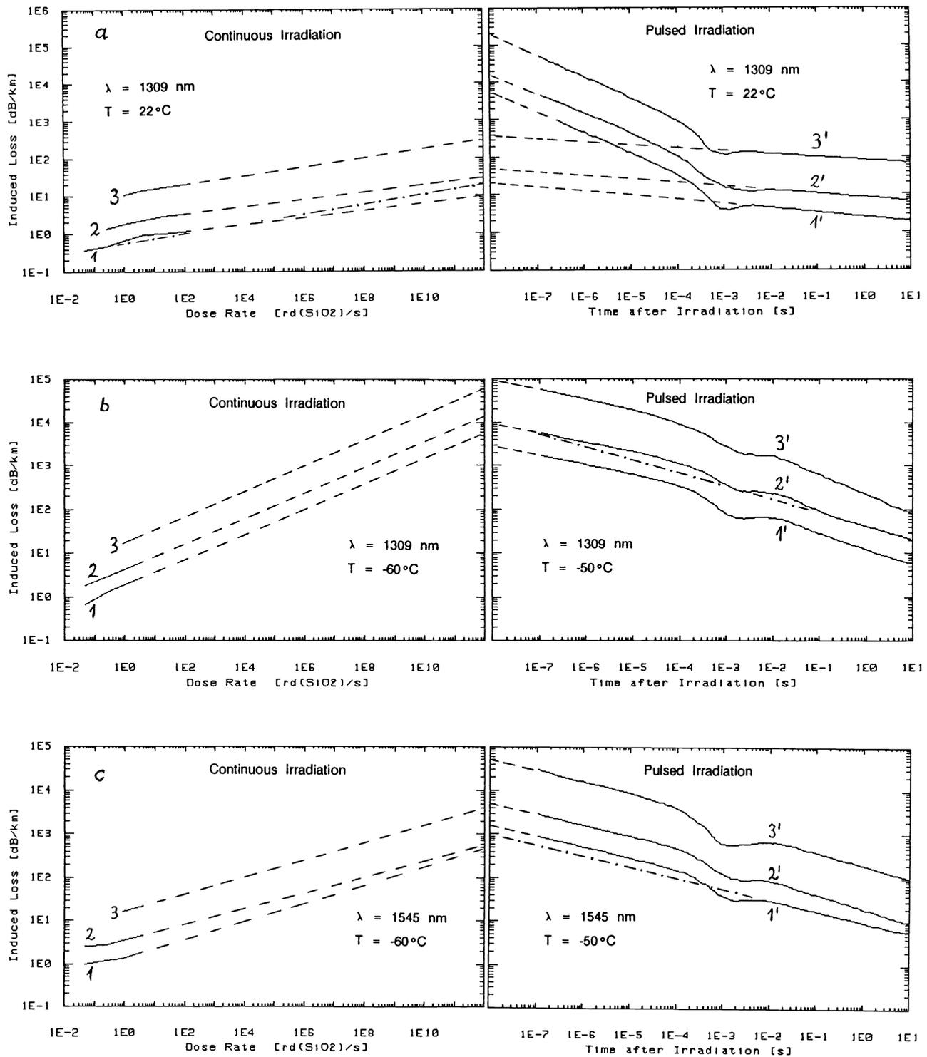
**Figures 4a-c:** Comparison of continuous and pulsed irradiation.  $D = 3 \cdot 10^3$  (rd) (1,1'),  $10^4$  rd (2,2'), and  $10^5$  rd (3,3'). Corresponding dose rates of the pulsed irradiations:  $\dot{D}_e = 10^{11}$  rd/s (1'),  $3 \cdot 10^{11}$  rd/s (2'), and  $3 \cdot 10^{12}$  rd/s (3').
