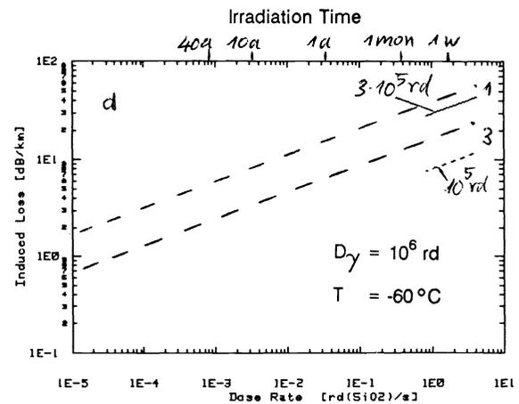
Figures 15a-d: Extrapolation of measured radiation induced losses to extremely low dose rates.
