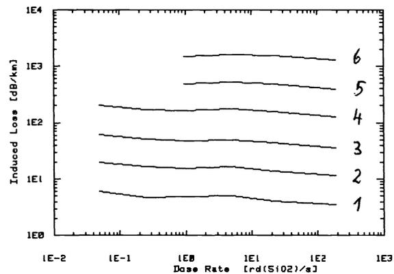
**Figure 10:** Induced loss as a function of dose rate.  $\lambda = 1308 \text{ nm}$ ,  $P \approx 10 \text{ } \mu\text{W}$ ,  $T = 22^\circ\text{C}$ .
