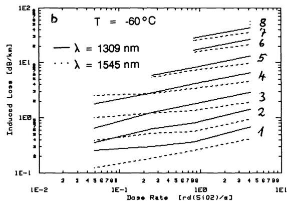
**Figures 3a,b:** Induced loss as a function of dose rate; Influence of temperature (a) and wavelength (b);  $P = 20 \mu\text{W}$ .
