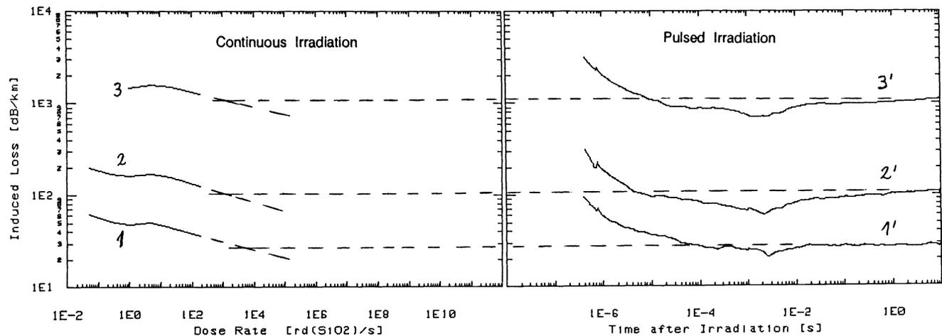
**Figure 11:** Comparison of continuous and pulsed irradiation.  $\lambda = 1308 \text{ nm}$ ,  $P \approx 10 \text{ } \mu\text{W}$ ,  $T = 22^\circ\text{C}$ .  $D = 3 \cdot 10^3 \text{ rd}$  (1,1'),  $10^4 \text{ rd}$  (2,2'), and  $10^5 \text{ rd}$  (3,3'). Corresponding dose rates of the pulsed irradiations:  $\dot{D}_e = 10^{11} \text{ rd/s}$  (1'),  $3 \cdot 10^{11} \text{ rd/s}$  (2'), and  $3 \cdot 10^{12} \text{ rd/s}$  (3').
