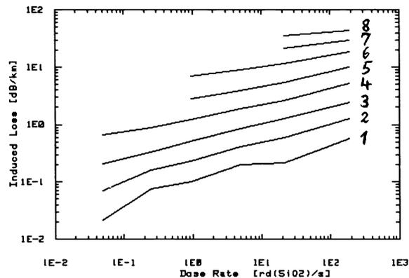
**Figure 7:** Induced loss as a function of dose rate.  $\lambda = 1308 \text{ nm}$ ,  $P \approx 10 \text{ } \mu\text{W}$ ,  $T = 22^\circ\text{C}$ .  $D = 300 \text{ rd}$  (1),  $10^3 \text{ rd}$  (2),  $3^7 10^3 \text{ rd}$  (3),  $10^4 \text{ rd}$  (4),  $3 \cdot 10^4 \text{ rd}$  (5),  $10^5 \text{ rd}$  (6),  $3 \cdot 10^5 \text{ rd}$  (7), and  $10^6 \text{ rd}$  (8).
