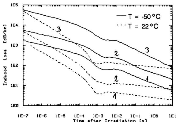
Figure 5: Induced loss after pulsed irradiation.  $P = 20 \mu\text{W}$ .
