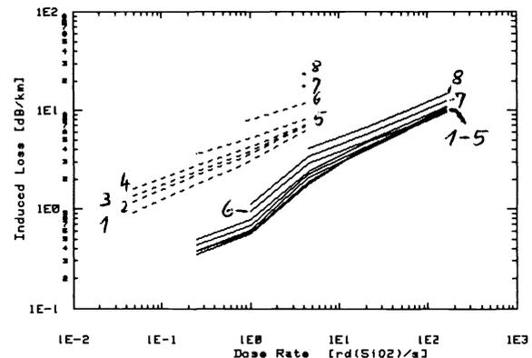
Figure 13: Induced loss as a function of dose rate.  $\lambda = 865$  nm,  $P = 10 \mu\text{W}$ ,  $D = 300$  rd (1),  $10^3$  rd (2),  $3 \cdot 10^3$  rd (3),  $10^4$  rd (4),  $3 \cdot 10^4$  rd (5),  $10^5$  rd (6),  $3 \cdot 10^5$  rd (7), and  $10^6$  rd (8).
